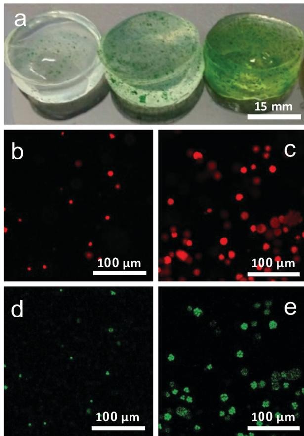
**Fig. 1** (a) Photograph showing the growth of algae cells within the alginate network over time (from left to right) at 1, 7 and 14 days of cultivation. (b–e) Confocal pictures show the growth of algae cells within alginate networks over time. (b) and (c) growth of algae after 1 and 14 days of cultivation using the fluorescence of the cell chloroplasts, respectively. (c) and (d) growth of algae after 1 and 14 days of cultivation using the fluorescein diacetate stain, respectively.
