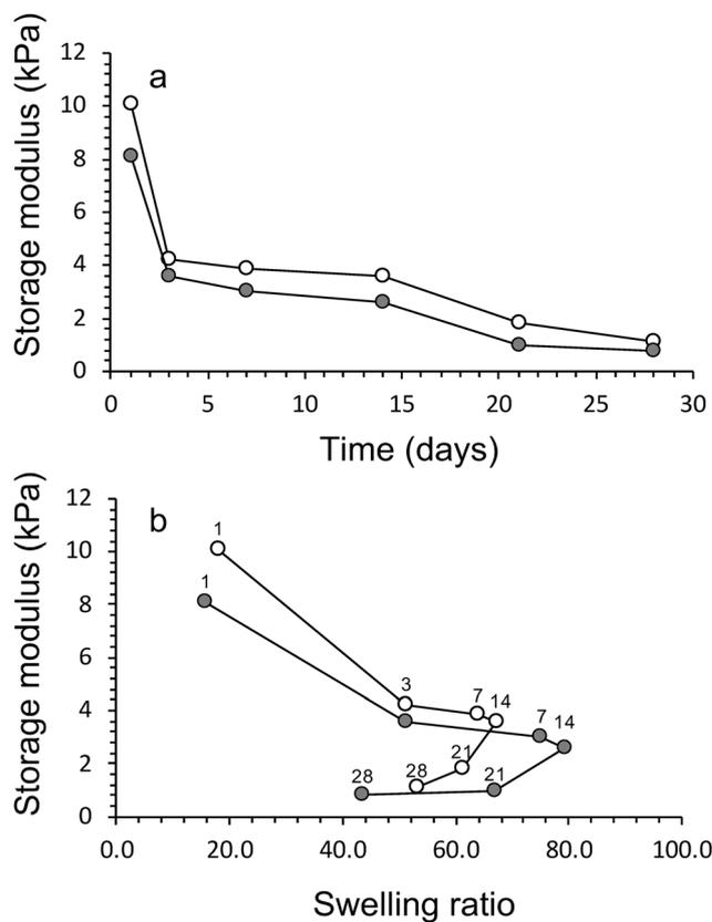
**Fig. 6** (a) Storage modulus values of alginate gels crosslinked with 0.05 M CaCl<sub>2</sub> (open spheres) and algae/alginate gels crosslinked with 0.05 M CaCl<sub>2</sub> (filled spheres) as a function of cultivation time. (b) Storage modulus values of alginate gels crosslinked with 0.05 M CaCl<sub>2</sub> (open spheres) and algae/alginate gels crosslinked with 0.05 M CaCl<sub>2</sub> (filled spheres) as a function of swelling ratio. Numbers indicate the days of cultivation time.
