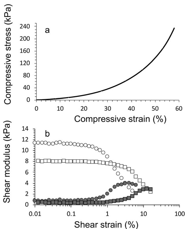
Fig. 5 (a) Compressive stress as a function of compressive strain for algae/alginate gels crosslinked with 0.05 M  $\text{CaCl}_2$  after 1 day of cultivation. (b) Shear modulus values of alginate gels crosslinked with 0.10 M  $\text{CaCl}_2$  (storage and loss modulus indicate by open and filled spheres, respectively) and algae/alginate gels crosslinked with 0.10 M  $\text{CaCl}_2$  (storage and loss modulus indicate by open and filled squares, respectively) after 1 day of cultivation.
