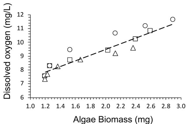
Fig. 3 Dissolved oxygen concentration as a function of algae biomass over 28 days of cultivation for algae/alginate gels (E1, spheres) crosslinked with 0.05 M  $\text{CaCl}_2$ , (E2, squares) 0.10 M  $\text{CaCl}_2$ , and (E3, triangles) 0.10 M  $\text{CaCl}_2$  with hydroxyapatite. Dashed line is a linear fit to the data.
