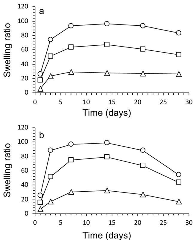
Fig. 4 Swelling ratios as a function of cultivation time. (a) alginate gels (spheres) crosslinked with 0.05 M  $\text{CaCl}_2$ , (squares) 0.10 M  $\text{CaCl}_2$ , and (triangles) 0.10 M  $\text{CaCl}_2$  with hydroxyapatite. (b) algae/alginate gels (E1, spheres) crosslinked with 0.05 M  $\text{CaCl}_2$ , (E2, squares) 0.10 M  $\text{CaCl}_2$ , and (E3, triangles) 0.10 M  $\text{CaCl}_2$  with hydroxyapatite.
