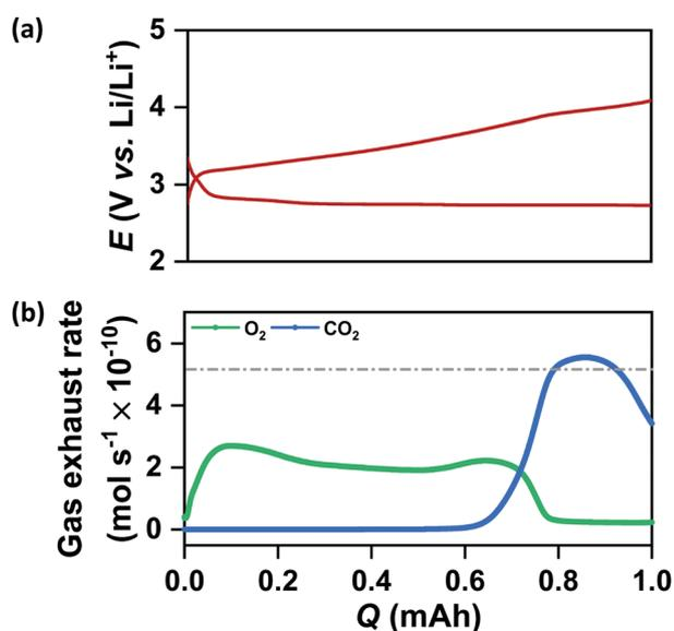
Fig. 5 (a) Galvanostatic DC/RC profiles of the mesoporous N-CMK-3-3 electrode in 1 M LiTFSI/tetraglyme electrolyte up to a fixed capacity of 1 mAh at  $100$  mA  $\text{g}^{-1}$  and (b) corresponding *in situ* gas evolution data during recharge of the cell.
