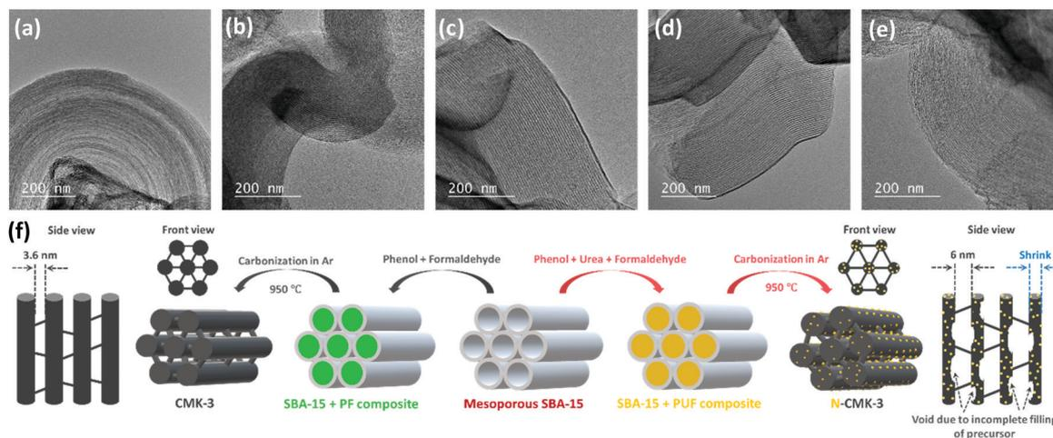
Fig. 3 Transmission electron microscopy (TEM) images of (a) CMK-3, (b) N-CMK-3-1, (c) N-CMK-3-2, (d) N-CMK-3-3 and (e) N-CMK-3-4. (f) Schematic representation of the synthetic steps for the mesoporous carbons.
