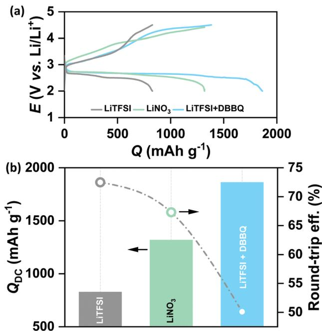
Fig. 2 (a) Galvanostatic DC/RC profiles of Li-air cells with a mesoporous CMK-3 electrode in different electrolytes and additives in the potential range of 2–4.5 V vs. Li/Li<sup>+</sup> at the same current density of 100 mA g<sup>-1</sup> and (b) comparison of DC capacity and round-trip efficiency of the cells in (a).
