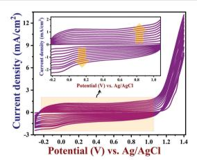
Fig. 1 The electrochemical polymerization of EDOT on GR/GCE from acetonitrile containing 0.01 M EDOT and 0.1 M lithium perchlorate at a scan rate of 0.05 V s<sup>-1</sup> (10 cycles) (inset: enlarged view).
