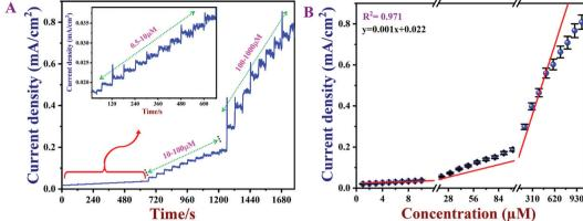
Fig. 9 (A) Amperometric response of PEDOT/GR/GCE for consecutive additions of nicotine (each 60 s) from  $0.5-1000 \mu M$  in 0.1 M PBS (pH 7) at an applied potential of +0.91 V. The electrolyte was stirred at 1000 rpm. (B) Calibration plot between the oxidation peak currents vs. the concentration of nicotine (n = 3).
