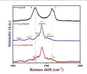
Fig. 4 Raman spectra of (a) GR, (b) PEDOT and (c) PEDOT/GR film (a 633 nm excitation laser was used).
