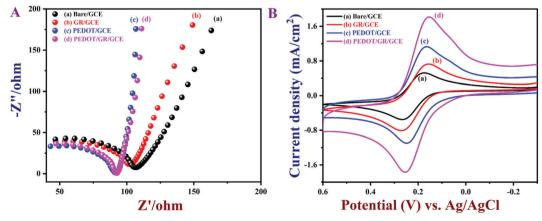
Fig. 5 (A) Nyquist plots and (B) CVs of bare/GCE, GR/GCE, PEDOT/GCE and PEDOT/GR/GCE in 0.1 M KCl containing 5 mM [Fe(CN)<sub>6</sub>]<sup>3-/4-</sup>. Scan rate =  $0.02 \text{ V s}^{-1}$
