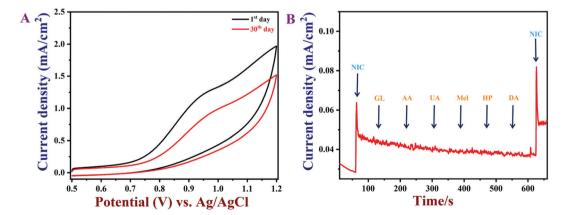
Fig. 11 (A) CVs of PEDOT/GR/GCE in 0.1 M PBS (pH 7) containing 100 μM nicotine with different storage times. (B) The amperometric response of PEDOT/GR/GCE with the additions of various interfering molecules (GL, AA, UA, Mel, HP, DA; concentration of each compound was 30 μM) with 5 μM of nicotine at an applied potential of +0.91 V. The PBS was stirred at 1000 rpm
