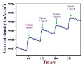
Fig. 10 Amperometric response of PEDOT/GR/GCE in 0.1 M PBS with successive addition of tobacco samples (real samples) containing different concentrations of nicotine at an applied potential of +0.91 V. The solution was stirred at a rate of 1000 rpm.
