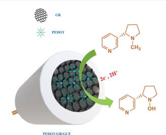
**Scheme 2** Electrochemical oxidation mechanism of nicotine on PEDOT/ GR/GCE.
