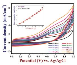
Fig. 7 Effect of scan rate on 100  $\mu$ M nicotine oxidation on PEDOT/GR/GCE (inset: the linear relationship between the oxidation peak current and square root of the scan rate (n=3)).
