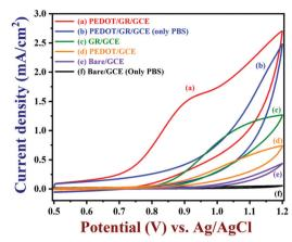
Fig. 6 CVs of PEDOT/GR/GCE (a), GR/GCE (c), PEDOT/GCE (d) and bare/ GCE (e) recorded in 0.1 M PBS (7 pH) with 100 µM nicotine. CVs of PEDOT/ GR/GCE (b) and bare/GCE (f) are shown in 0.1 M PBS (7 pH) without nicotine (scan rate =  $0.02 \text{ V s}^{-1}$ ).
