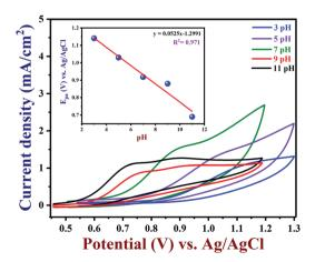
**Fig. 8** Effect of pH on the oxidation of 100  $\mu$ M nicotine in 0.1 M PBS with various pH (from 3 to 11) on a PEDOT/GR/GCE at a scan rate of 0.02 V s<sup>-1</sup> (inset: a linear plot of the  $E_{pa}$  of nicotine oxidation vs. pH).
