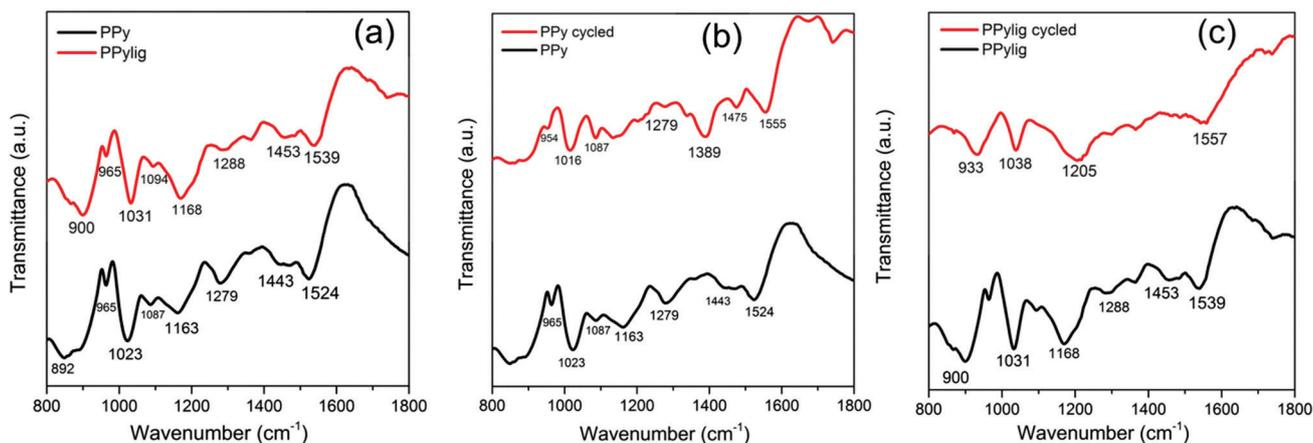
**Fig. 6** (a) IR spectra of the electrodeposited polypyrrole (black line) and polypyrrole–lignin composite (red line), (b) comparison of polypyrrole (black line) and polypyrrole after cycling in a Zn-ion battery (red line) and (c) comparison of the polypyrrole–lignin composite (black line) and polypyrrole–lignin composite after cycling in a Zn-ion battery (red line).
