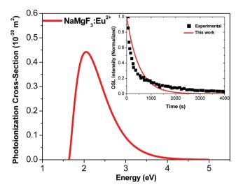
**Fig. 6** Photoionization cross-section *versus* electromagnetic radiation energy for NaMgF $_3$ :Eu $^{2+}$ . Inset shows experimental data from ref. 77 and theoretical OSL decay patterns for NaMgF $_3$ :Eu $^{2+}$ . The experimental decay curve was obtained after irradiation with an X-ray dose of 219 mGy. 77
