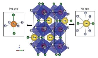
Fig. 1 The crystalline structure of NaMgF<sub>3</sub> in an orthorhombic lattice with space group Pbnm. Na and Mg sites are shown in detail.
