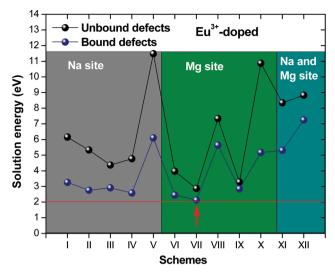
Fig. 2 Solution energies of bound and unbound defects for incorporation of  ${\rm Eu^{3+}}$  into  ${\rm NaMgF_3}.$
