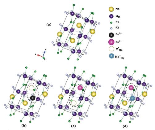
$\begin{array}{ll} \text{Fig. 4} & \text{Illustration of } Eu^{3+} \text{ and } Eu^{2+} \text{ incorporation into } NaMgF_3 \text{ with the most favourable charge compensation mechanism: (a) pure } NaMgF_3, \text{ (b)} \\ \left(Eu^{\bullet}_{Mg} + V'_{Na}\right) \text{ cluster, (c) } \left(Eu^{\bullet}_{Na} + V'_{Na}\right) \text{ cluster, and (d) } \left(Eu^{\bullet}_{Na} + Na'_{Mg}\right) \text{ cluster.} \end{array}$
