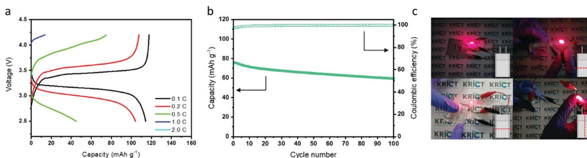
**Fig. 5** (a) Charge-discharge profile of the graphite/LiFePO<sub>4</sub> full-cell with the BisA-PEGDME polymer electrolyte including FEC at various C-rates. (b) Cycle stability of graphite/LiFePO<sub>4</sub> full-cell at  $0.5 \text{ C}$ . (c) Flexibility test of the graphite/LiFePO<sub>4</sub> pouch cell with the BisA-PEGDME polymer electrolyte.
