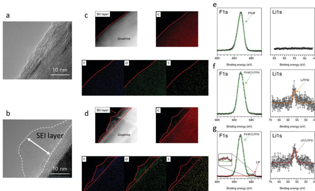
**Fig. 2** Transmission electron microscopy (TEM) image of graphite (a) without and (b) with FEC after the first cycle. EDS mapping images of graphite (c) without and (d) with FEC after the first cycle. X-ray photoelectron spectroscopy (XPS) spectra of the graphite electrode: (e) pristine, (f) without FEC after the first cycle, and (g) with FEC after the first cycle. A lithium/graphite half-cell with PEGDME electrolyte was fabricated, and the cell was run for one lithiation/delithiation cycle.
