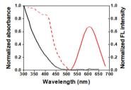
Fig. 2 Spectroscopic characterization of the GSH-AuNCs: the absorption (solid, black), emission (solid, red) ( $\lambda_{ex}$  = 375 nm), and excitation (dash, red) spectra.
