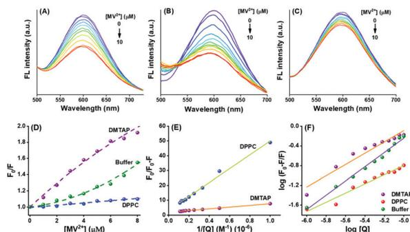
Fig. 4 Quenching of the fluorescence from GSH-AuNCs by the  $MV^{2+}$  ions in aqueous buffer (pH 7.4) in (A) the absence of lipids, (B) and (C) the presence of the DMTAP and DPPC GUVs. The various plots with modified Stern–Volmer equations are given in (D) to (F) to obtain the different physical parameters arising due to the interactions as explained in the text.
