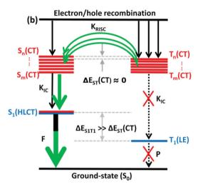
**Fig. 6** A simple scheme of (a) the traditional "Hot exciton" mode and (b) the multi-channel "Hot exciton" mode in the electroluminescence process. Here, F: fluorescence; P: phosphorescence.
