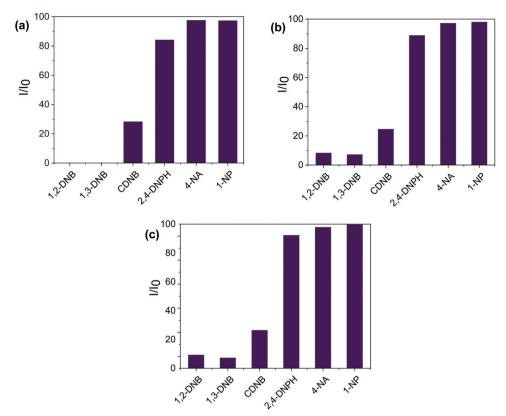
PL quenching efficiency of different analytes in the presence of (a) LCo-1; (b) L-Zn; and (c) LCo-2 respectively for 200 μL analyte volume.
