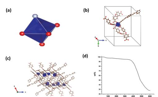
Fig. 3 (a) The SBU unit of the LCo-2 MOF with color code blue: central atom (Co), red: oxygen atoms and indigo blue: nitrogen; (b) complete structure of the SBU with coordinating molecules bpeb and oba; (c) 3-dimensional structure, and (d) thermogravimetric curve of the LCo-2 MOF.
