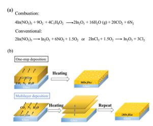
Fig. 6 (a) Chemical formulas of combustion and classical (nitrate- and chloride-routes) reactions to obtain  $In_2O_3$  thin films. (b) Schematic diagram of the influence of gaseous products on porosity in one-step- and multilayer-deposited films.
