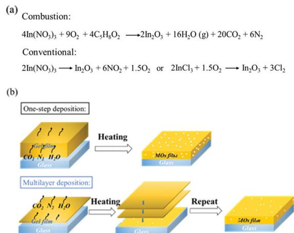
Fig. 6 (a) Chemical formulas of combustion and classical (nitrate- and chloride-routes) reactions to obtain  $\text{In}_2\text{O}_3$  thin films. (b) Schematic diagram of the influence of gaseous products on porosity in one-step- and multilayer-deposited films.
