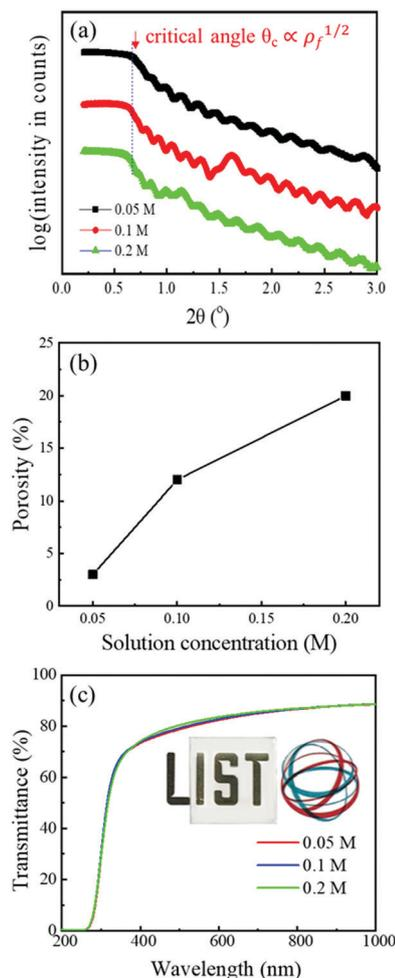
**Fig. 3** (a) XRR patterns of ITO thin films prepared from solutions with different concentrations. (b) Extracted porosity of the films as a function of solution concentration. (c) Optical transmittance of the films. In (b) lines between the experimental points are guides to the eyes. In (c) the inset shows visual appearance of ITO-coated glass.
