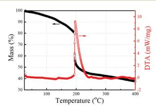
Fig. 1 TGA (black symbols) and DTA (red symbols) curves of the dried 0.05 M solution.
