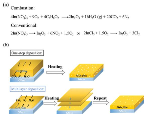
Fig. 6 (a) Chemical formulas of combustion and classical (nitrate- and chloride-routes) reactions to obtain In<sub>2</sub>O<sub>3</sub> thin films. (b) Schematic diagram of the influence of gaseous products on porosity in one-step- and multilayer-deposited films.
