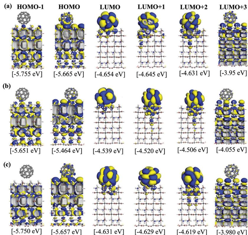
Fig. 4 Calculated Kohn–Sham orbitals and energy eigenvalues of a MAPbI<sub>3</sub>/C<sub>60</sub> heterojunction with tetragonal MAPbI<sub>3</sub> from HOMO–1 to LUMO+3 levels. Yellow and blue denote plus and minus regions of the orbitals. The perovskite has a topC geometry with a fullerene C<sub>60</sub> on the (a) aboveC, (b) above and (c) bridge positions.
