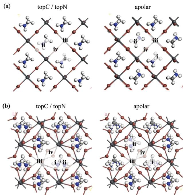
Fig. 3 Position of a fullerene C<sub>60</sub> on (a) cubic and (b) tetragonal MAPbI<sub>3</sub>(001) surfaces with MAI terminations for topC/topN and apolar geometries: (i) aboveC, (ii) aboveN, (iii) aboveI, and (iv) bridge. H, C, N, I, and Pb atoms are represented by the white, light grey, blue, brown, and dark grey spheres, respectively. H, C, N, I, and Pb atoms are represented by the white, light grey, blue, brown, and dark grey spheres, respectively.
