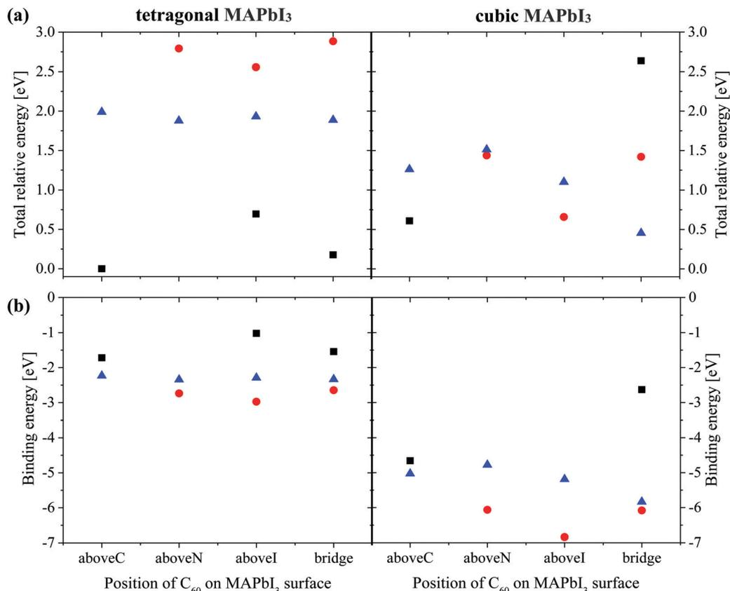
Fig. 5 (a) Total DFT-D and (b) binding energies of a MAPbI<sub>3</sub>/C<sub>60</sub> heterojunction relative to the topC-aboveC configuration. Orientations of the MA cation with respect to the (001) surface are: topC (black), topN (red) and apolar (blue).
