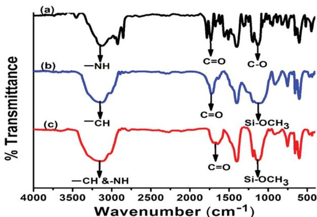
Fig. 2 FTIR spectrum of DMPM (a), poly(MPTS) (b) and poly(DMPM-co-MPTS) (c).
