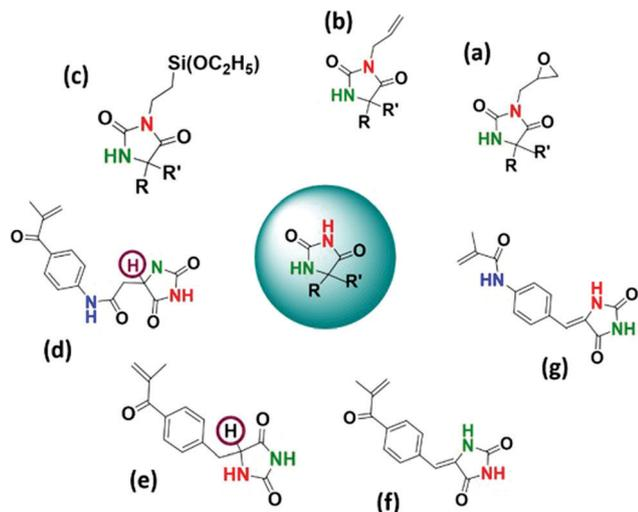
**Scheme 1** Hydantoin monomers with lost imide position for Cl binding (a–c), monomers containing tertiary hydrogen that can prompt the release of HCl after chlorination (d and e), a stable monomer with 2 Cl binding sites (f) and a stable monomer with 3 Cl binding sites (g).
