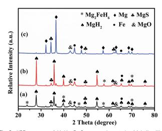
Fig. 8 XRD patterns of MgH $_2$ -Fe $_7$ S $_8$  composites at the (a) ball-milling (b) hydrogenation (c) dehydrogenation stages.
