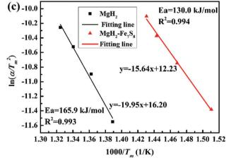
Fig. 4 DSC curves of (a) pure MgH $_2$  and (b) MgH $_2$  + 16.7 wt% Fe $_7$ S $_8$  composites with a heating rate of 5 K min $^{-1}$ , 10 K min $^{-1}$ , 15 K min $^{-1}$ . (c) The corresponding Kissinger plots for the hydrogen desorption reaction for MgH $_2$  and MgH $_2$  + 16.7 wt% Fe $_7$ S $_8$  composites at various heating rates.
