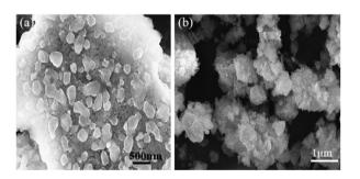
Fig. 7 SEM images of (a) MgH  $_2$  , (b) MgH  $_2\text{--}\text{Fe}_7\text{S}_8$  composite after the re-hydrogenation process.
