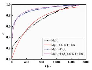
Fig. 6 Fitted hydrogenation kinetic curves of  $MgH_2$  and  $MgH_2 + 16.7$  wt%  $Fe_7S_8$  composites at 523 K under the pressure of 3 MPa.
