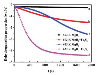
Fig. 3 Dehydrogenation properties of MgH $_2$  and MgH $_2$  + 16.7 wt% Fe $_7$ S $_8$  composite at 573 K, 623 K.
