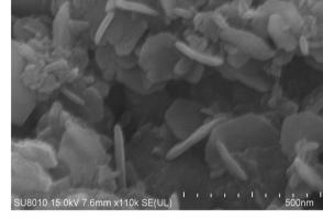
Fig. 1 (a) XRD pattern of the as-synthesized  $Fe_7S_8$  (b) SEM image of the as-synthesized  $Fe_7S_8$ .
