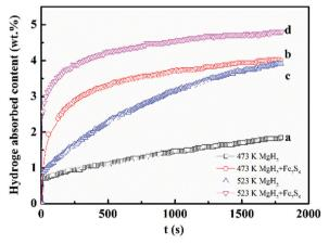
Fig. 5 Hydrogenation properties of (a) MgH $_2$  at 473 K; (b) MgH $_2$  + 16.7 wt% Fe $_7$ S $_8$  composite at 473 K; (c) MgH $_2$  at 523 K; (d) MgH $_2$  + 16.7 wt% Fe $_7$ S $_8$  composite at 523 K.
