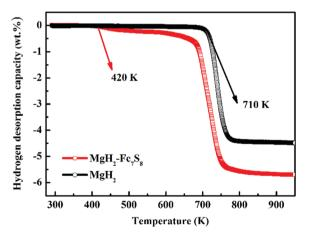
Fig. 2 Thermal decomposition curves of  ${\rm MgH_2}$  and  ${\rm MgH_2}$  + 16.7 wt%  ${\rm Fe_7S_8}$  composite.
