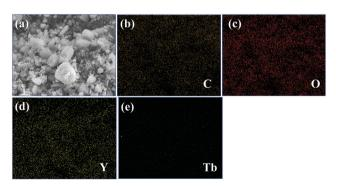
Fig. 3 (a) SEM image in which elemental mapping is performed in  $\bf 1a$  and elemental mapping images, (b) C K, (c) O K, (d) Y L and (e) Tb L.
