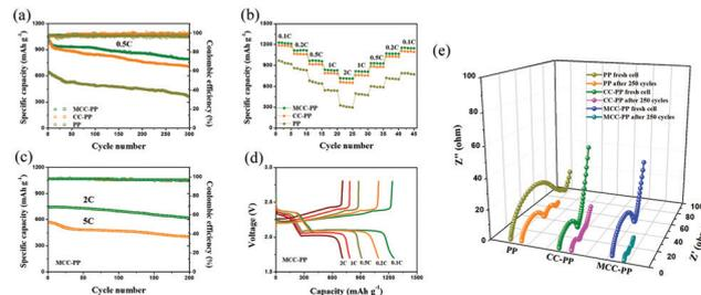
**Fig. 2** Electrochemical characterization of batteries with different interlayers. (a) Cycling performances (0.5 C) and (b) rate capabilities of batteries with PP, CC–PP and MCC–PP; (c) cycling performances of batteries with MCC–PP at 2 C and 5 C; (d) initial galvanostatic charge–discharge profiles of batteries with MCC–PP at various current rates; (f) EIS curves of batteries with PP, CC–PP and MCC–PP.
