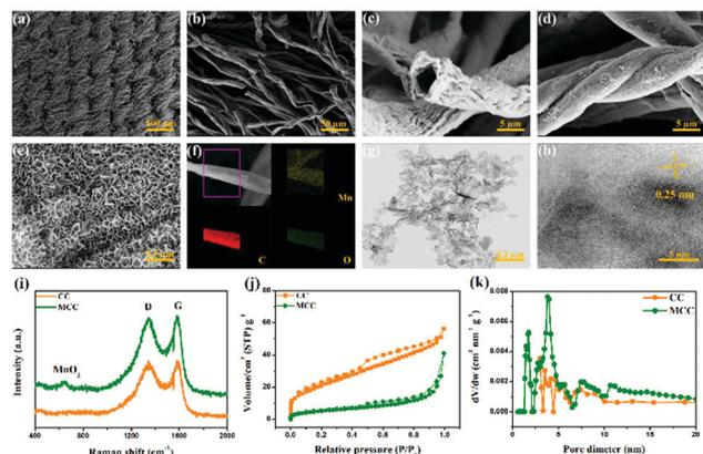
**Fig. 1** Scanning electron microscopy (SEM) images of carbon cloth (a–c) and the MCC composite (d and e); elemental mapping images (f) of Mn, C, and O in the MCC composite; transmission electron microscopy (TEM) (g) and high resolution TEM (HRTEM) images (h) of MnO<sub>2</sub>; (i) Raman spectra of CC and MCC composites; nitrogen adsorption–desorption isotherms (j) and pore size distributions (k) of CC and MCC composites.
