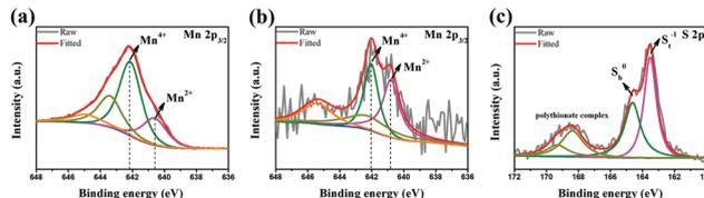
Fig. 3 Mn 2p<sub>3/2</sub> XPS spectra of MCC composites (a) before and (b) after soaking tests; (c) the S 2p XPS spectrum of MCC composites after the soaking tests.
