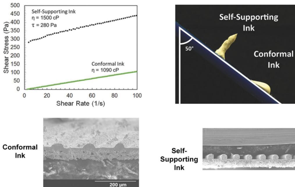
Fig. 16 Comparison between the self-supporting and conformal inks formulated by McOwen *et al.*<sup>90</sup> (adapted with permission from ref. 90, Copyright 2018 John Wiley and Sons).
