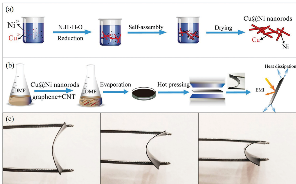
Fig. 1 Schematic illustration of the fabrication process of (a) Cu@Ni nanorods and (b) the PVDF/CNT/graphene/Cu@Ni composite film and (c) the digital image of the bent composite film with 8 wt% Cu@Ni.
