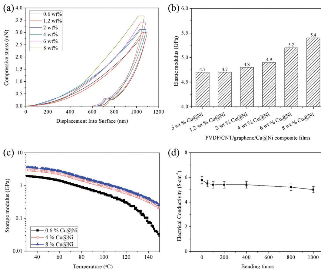
**Fig. 8** (a) Compression versus displacement curve and (b) the elastic modulus of the composite films obtained using a nano-indenter; (c) storage modulus of the films as a function of temperature; (d) EC with 8 wt% Cu@Nis after repeated bending.
