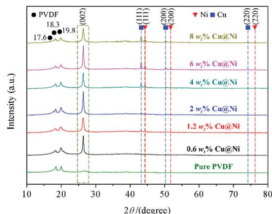
Fig. 2 XRD patterns of the PVDF/CNT/graphene/Cu@Ni composite films.
