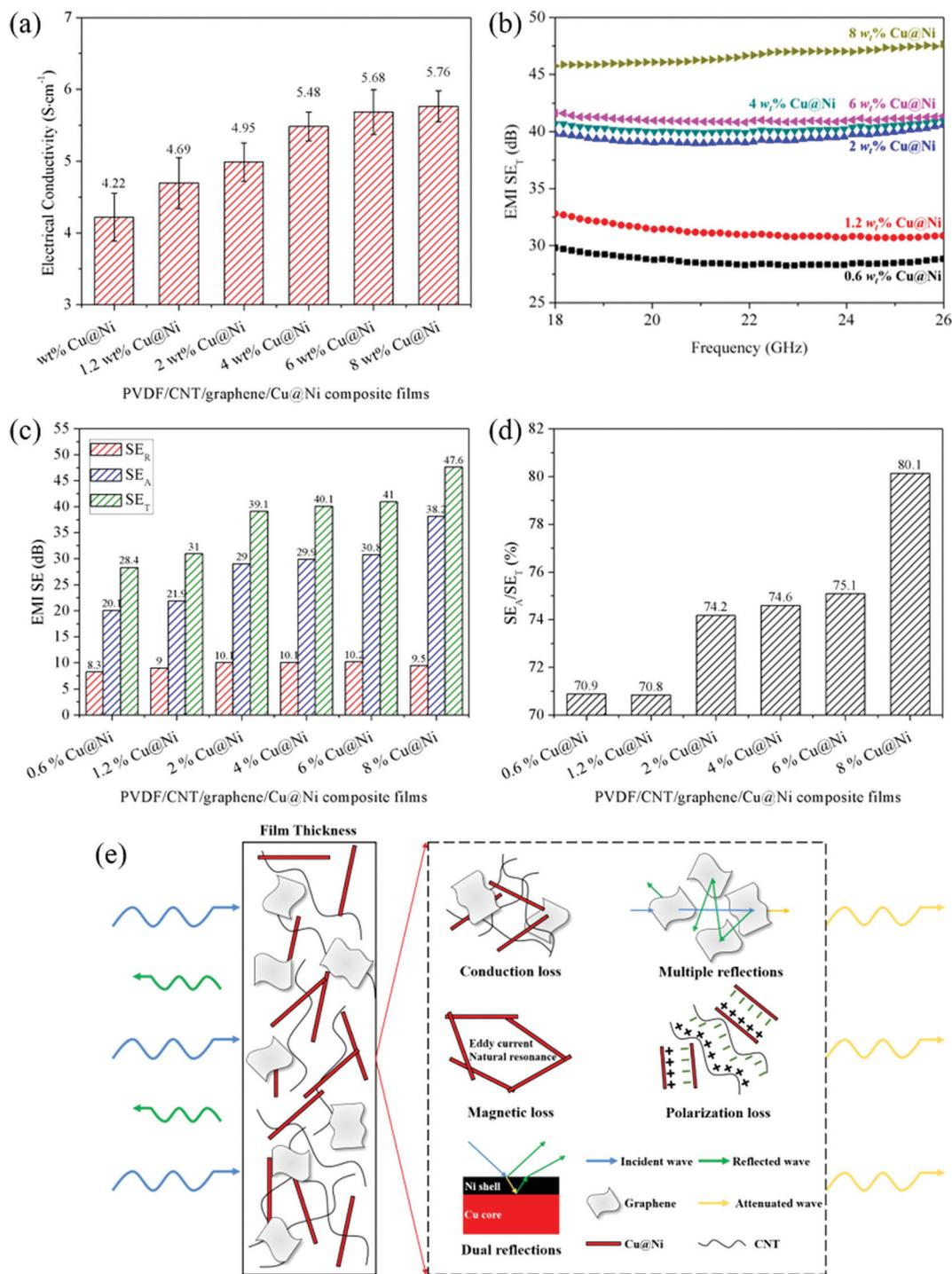
Fig. 5 (a) EC of the PVDF/CNT/graphene/Cu@Ni composite films; (b) EMI SE of the composite films at a frequency from 18 GHz to 26 GHz; (c) the SE (SE<sub>R</sub>, SE<sub>A</sub> and SE<sub>T</sub>) and (d) the ratios of SE<sub>A</sub>/SE<sub>T</sub> for the composite films at a frequency of 22 GHz; and (e) schematic EMI shielding mechanisms for the composite film.
