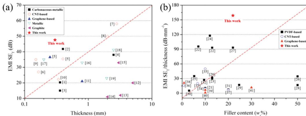
Fig. 6 Comparison of (a) EMI SE and (b) EMI SE/ $t$  of PVDF/CNT/graphene/Cu@Ni composite films with those in the literature. The numbers inside the panel are the reference numbers listed in Tables S2 and S3 in the ESI,<sup>†</sup> respectively.
