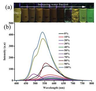
Fig. 2 (a) Digital images and (b) fluorescence spectra of 3 at different water fraction in CH<sub>3</sub>CN:water in day 2.  $\lambda_{exc}$  = 365 nm (for the digital images) and 370 nm (for the spectra).
