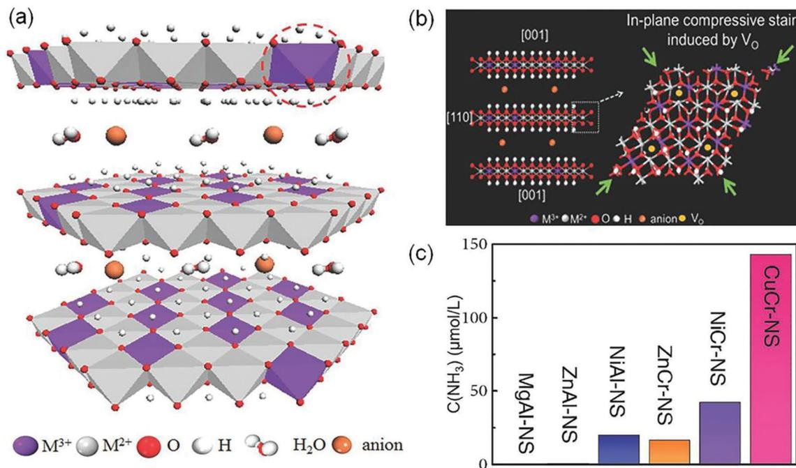
Fig. 4 (a) Schematic representation of the layered LDH structure with defective  $MO_6$  octahedra. (b) Schematic of the in-plane biaxial compressive strain induced by  $V_O$ . (c) The yield of  $NH_3$  over different LDH photocatalysts under visible-light illumination ( $\lambda > 400 \text{ nm}$ ). Reproduced from ref. 34 with permission from Wiley-VCH.
