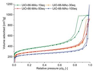
Fig. 3 N<sub>2</sub> sorption isotherms of UiO-66-MAc-10 eq., 30 eq., 50 eq. and 100 eq. at 77 K. Filled symbols: adsorption; empty symbols: desorption.
