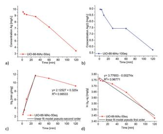
Fig. 5 Time-dependent removal of Aq(ı) by UiO-66-MAc-50 eq. (a) and UiO-66-MAc-100 eq. (b) from a starting  $Ag^+$  concentration of 10 mg  $L^{-1}$ . Linear fit for pseudo second-order kinetics (c) and for pseudo first-order kinetics (d) for the uptake in UiO-66-MAc-50 eq. See Fig. S48, ESI† for the linear fits for the uptake in UiO-66-MAc-100 eq.
