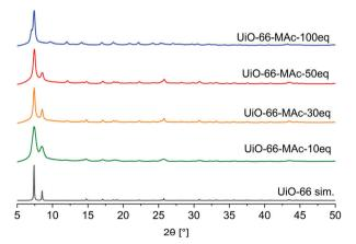
Fig. 1 PXRD patterns of UiO-66-MAc with different HMAc equivalents used in the synthesis and simulated diffractogram of UiO-66 (from CIF CCDC 837796).<sup>52</sup>
