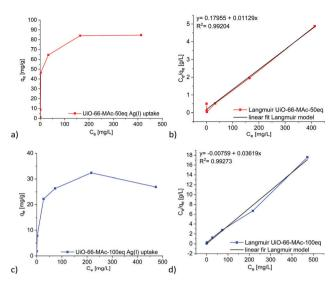
Fig. 4 Isotherms of the Ag(ı) removal with UiO-66-MAc-50 eq. (a) and UiO-66-MAc-1000 eq. (c) ( $q_e$  = uptake at equilibrium;  $c_e$ = concentration at equilibrium). (b and d) Correlated fitted equilibrium data by the linearized Langmuir adsorption model.
