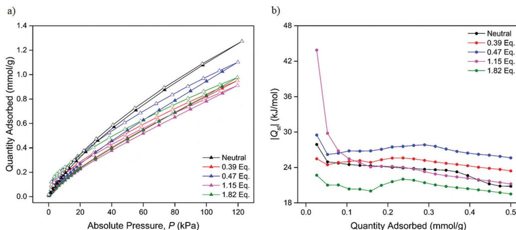
**Fig. 5** (a) CO<sub>2</sub> adsorption (closed triangles) and desorption (open triangles) isotherms of the neutral and samples reduced by 0.39, 0.47, 1.15 and 1.82 equiv. of LiNP at 298 K and (b) CO<sub>2</sub> isosteric heat of adsorption profiles for the neutral and chemically reduced samples.
