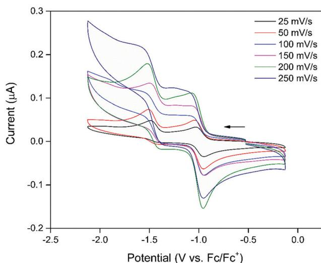
Fig. 1 CV of **1** in 0.1 M  $[(n\text{-C}_4\text{H}_9)_4\text{N}]\text{PF}_6/\text{DMF}$  supporting electrolyte at scan rates of 25–250  $\text{mV s}^{-1}$ . The arrow indicates the direction of the forward scan.
