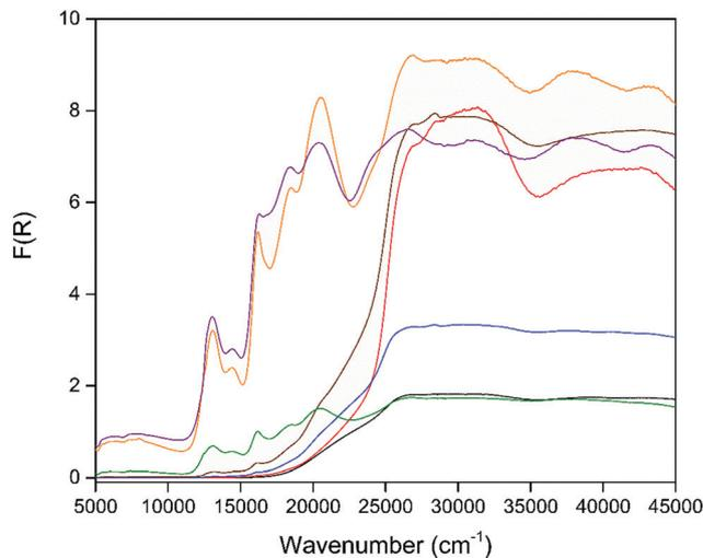
**Fig. 4** Solid-state UV/Vis/NIR spectra of [Zn<sub>2</sub>(DSNDI)], **1** (black) and its reduced analogues generated by chemical reduction with 0.39 (red), 0.47 (blue), 1.15 (brown), 1.82 (green), 2.27 (orange) and 2.83 equiv. (purple) of LiNP.
