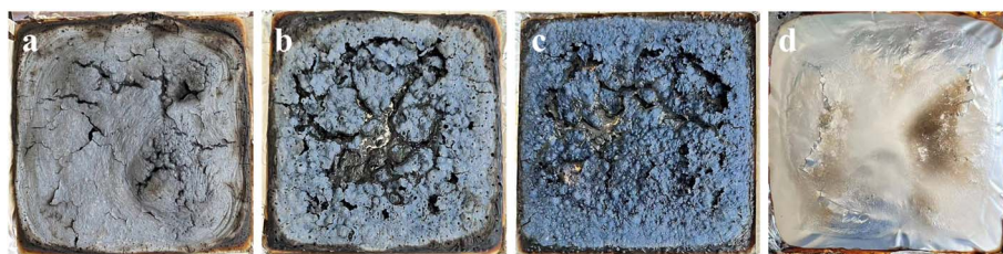
Fig. 10 Digital images of the char residues of EVA/MHx60 (a), EVA/MHy60 (b), EVA/MHz60 (c), and pure EVA (d).
