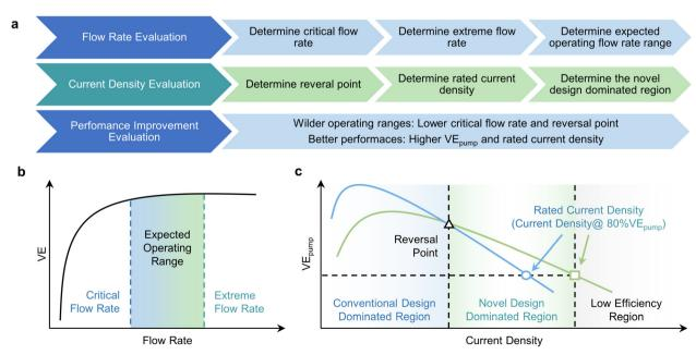
Fig. 8 (a) The basic approaches for evaluation. (b) The overall trend of VE and the determination of operating flow rates. (c) The overall trend of VE pump and the determination of operating current densities.
