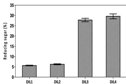
Fig. 3 Yields of reducing sugars. DIL1:  $[\text{PF}_6][(\text{PYR})\text{C}_4(\text{MIM})][\text{Br}]$ ; DIL2:  $[\text{PF}_6][(\text{PYR})\text{C}_5(\text{MIM})][\text{Br}]$ ; DIL3:  $[\text{PF}_6][(\text{PYR})\text{C}_4(\text{IMCH}_2\text{COOH})][\text{Br}]$ ; DIL4:  $[\text{PF}_6][(\text{PYR})\text{C}_5(\text{IMCH}_2\text{COOH})][\text{Br}]$ .
