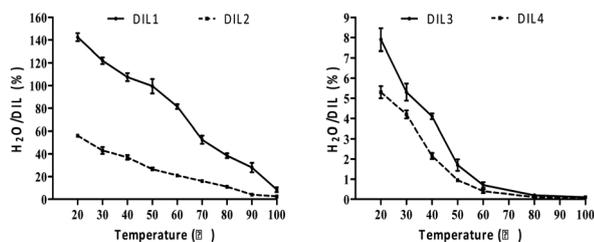
Fig. 2 Miscibility of DILs with water. DIL1:  $[\text{PF}_6][(\text{PYR})\text{C}_4(\text{MIM})][\text{Br}]$ ; DIL2:  $[\text{PF}_6][(\text{PYR})\text{C}_5(\text{MIM})][\text{Br}]$ ; DIL3:  $[\text{PF}_6][(\text{PYR})\text{C}_4(\text{IMCH}_2\text{COOH})][\text{Br}]$ ; DIL4:  $[\text{PF}_6][(\text{PYR})\text{C}_5(\text{IMCH}_2\text{COOH})][\text{Br}]$ .
