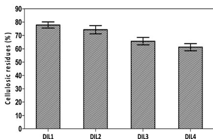
Fig. 4 Yields of cellulosic residues. DIL1:  $[\text{PF}_6][(\text{PYR})\text{C}_4(\text{MIM})][\text{Br}]$ ; DIL2:  $[\text{PF}_6][(\text{PYR})\text{C}_5(\text{MIM})][\text{Br}]$ ; DIL3:  $[\text{PF}_6][(\text{PYR})\text{C}_4(\text{IMCH}_2\text{COOH})][\text{Br}]$ ; DIL4:  $[\text{PF}_6][(\text{PYR})\text{C}_5(\text{IMCH}_2\text{COOH})][\text{Br}]$ .
