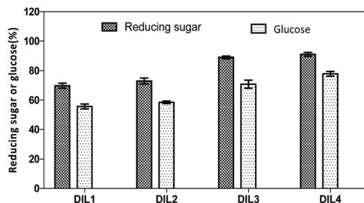
Fig. 5 Yields of reducing sugars and glucose. DIL1:  $[\text{PF}_6][(\text{PYR})\text{C}_4(\text{MIM})][\text{Br}]$ ; DIL2:  $[\text{PF}_6][(\text{PYR})\text{C}_5(\text{MIM})][\text{Br}]$ ; DIL3:  $[\text{PF}_6][(\text{PYR})\text{C}_4(\text{IMCH}_2\text{COOH})][\text{Br}]$ ; DIL4:  $[\text{PF}_6][(\text{PYR})\text{C}_5(\text{IMCH}_2\text{COOH})][\text{Br}]$ .
