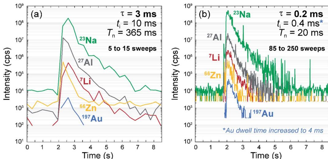
**Fig. 1** Transient time-resolved LA-ICP-MS signals of two single shot analyses (60  $\mu\text{m}$  laser spot) in NIST SRM610 glass using two different timing setups: (a) long and (b) short settling ( $\tau$ ), dwell ( $t_i$ ) and sweep ( $T_n$ ) times. Intensities for a total of 28 analytes were acquired in both cases (amu 7, 11, 23, 25, 27, 29, 34, 35, 39, 43, 55, 57, 63, 66, 75, 79, 85, 88, 95, 107, 121, 133, 137, 140, 197, 208, 209, 238), only 5 are shown.
