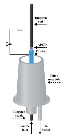
Fig. 1 A schematic drawing of the developed FLC APGD systems.
