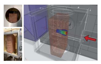
Fig. 2 The visualization of the calculated capture rate field for the 25 mm position of the pavement stone (Pos A), with a vertical cutting plane at the beam center. Neutrons reach the sample from the right, as shown by the red arrow. Additional plots are shown in ESI 3.†
