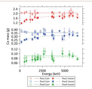
Fig. 6 The corrected (open symbols) and uncorrected (closed symbols) masses of the element Ca in the active measurement volume. The corrected mass values from analytical peaks at various gamma energies show no energy-dependent tendency and agree within the 1-sigma statistical uncertainty, calculated as described in ref. 24. The interpolation curves were determined with a nonlinear weighted least-squares fit.
