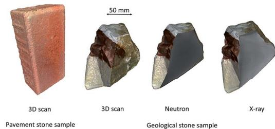
**Fig. 1** The textured 3D surface mesh of the pavement stone validation object as well as the stone geological object. The neutron and X-ray tomograms of the latter are also shown after registration in VGStudio MAX. The CT data cuts revealed no internal structures. The 3D photorealistic digital models of the measured objects are available as ESI 1 and 2.†
