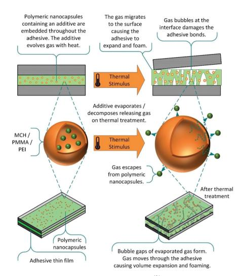
Scheme 11 Thermally induced debonding via evaporable and decomposable additives. 124
