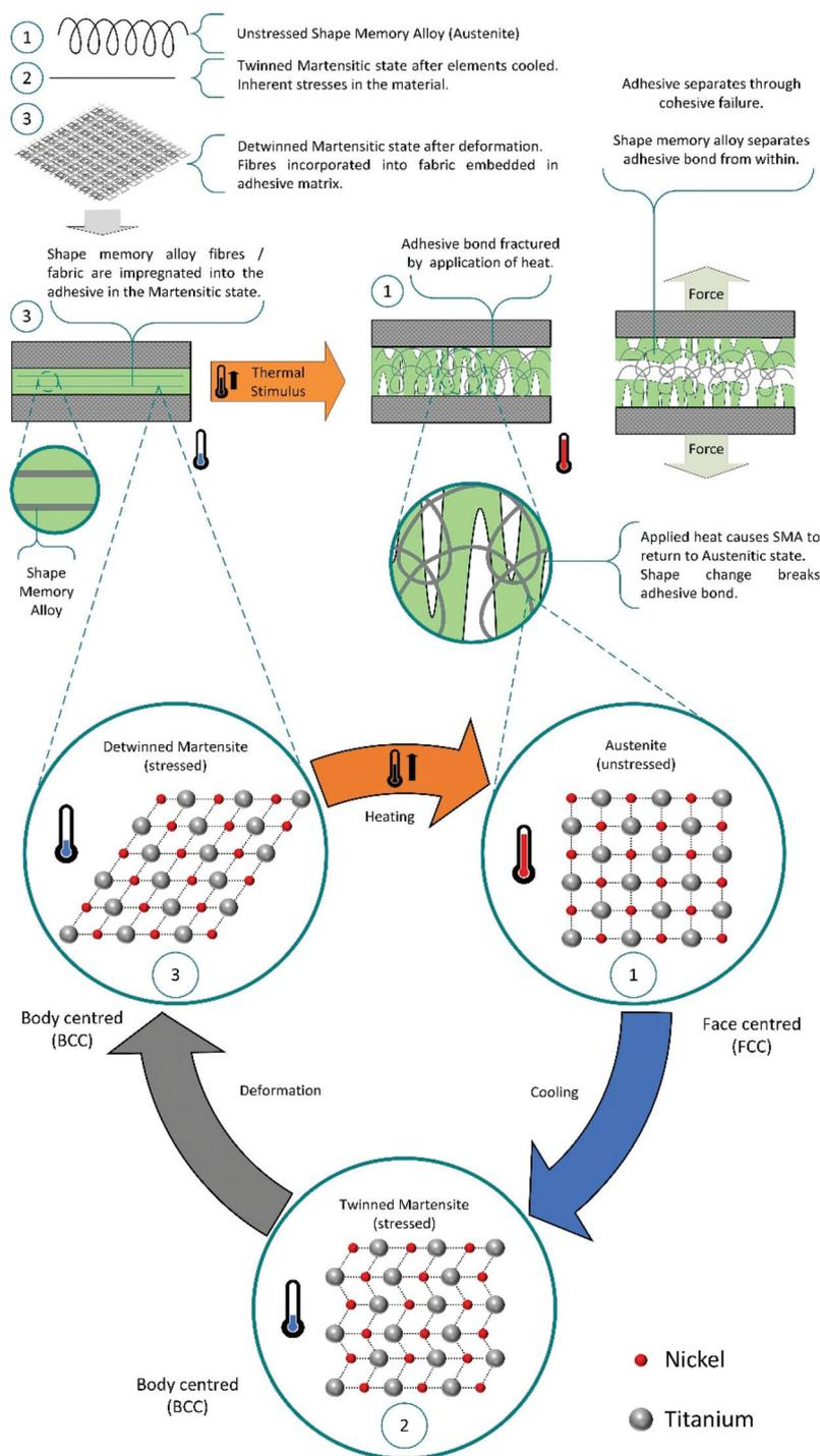
**Scheme 12** Schematic representation of the debonding mechanism using shape memory additives.
