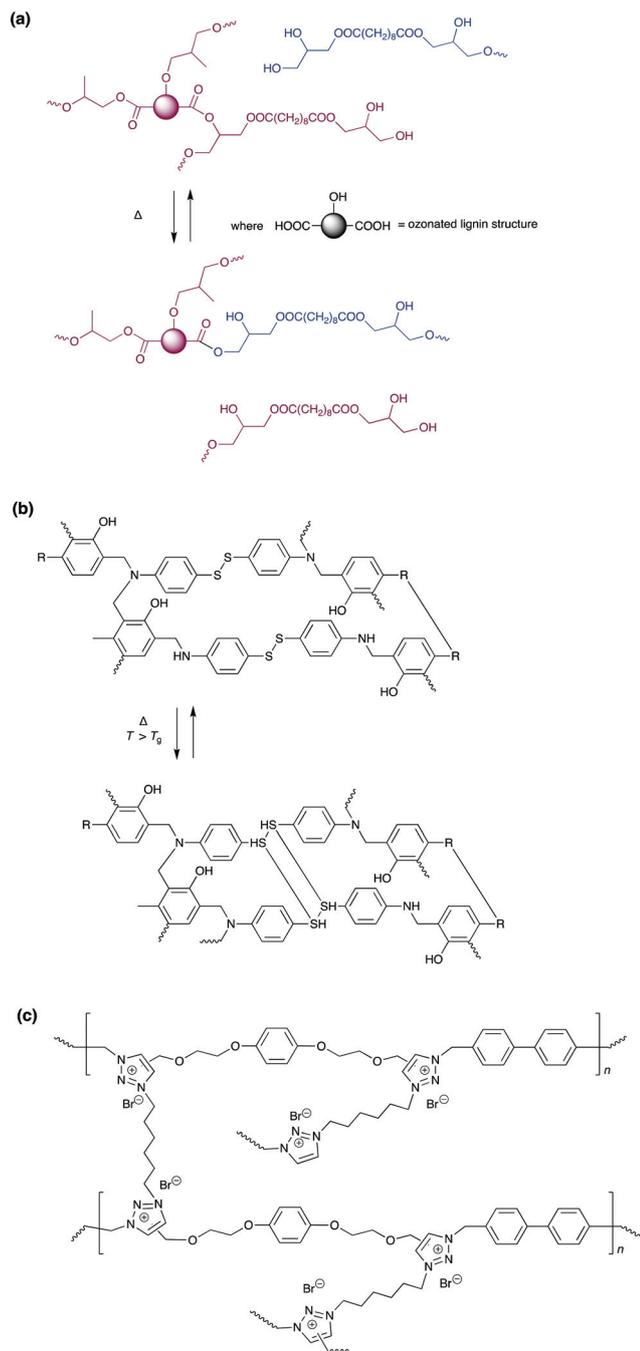
**Scheme 15** Simplified cross-linked network and mechanism of chemical bond re-arrangement upon heating in (a) lignin-based vitrimer containing  $\beta$ -hydroxyester linkages;<sup>194</sup> (b) poly(benzoxazine) vitrimer containing disulfide bonds,<sup>203</sup> and (c) poly(1,2,3-triazolium) vitrimers which display reversible adhesion.<sup>206</sup>
