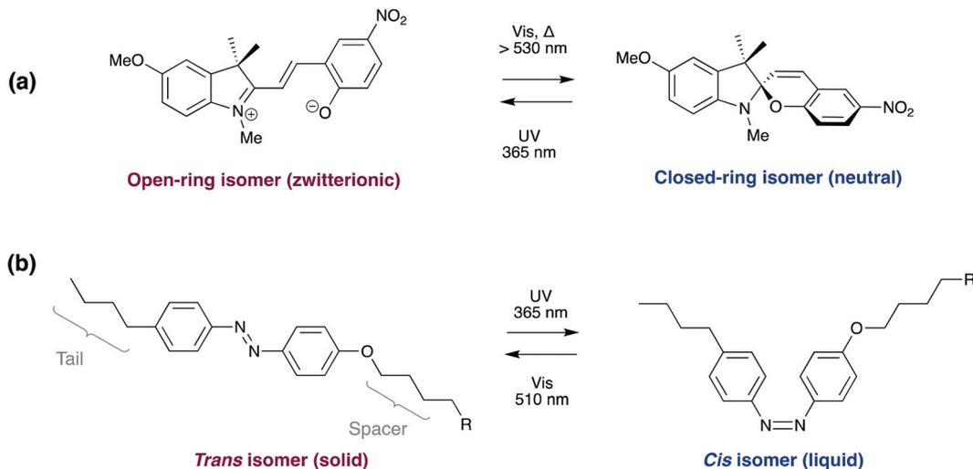
**Scheme 6** Photo-induced isomerisation of (a) spiropyran and (b) azobenzene derivatives, utilised in reversibly bonding adhesives.
