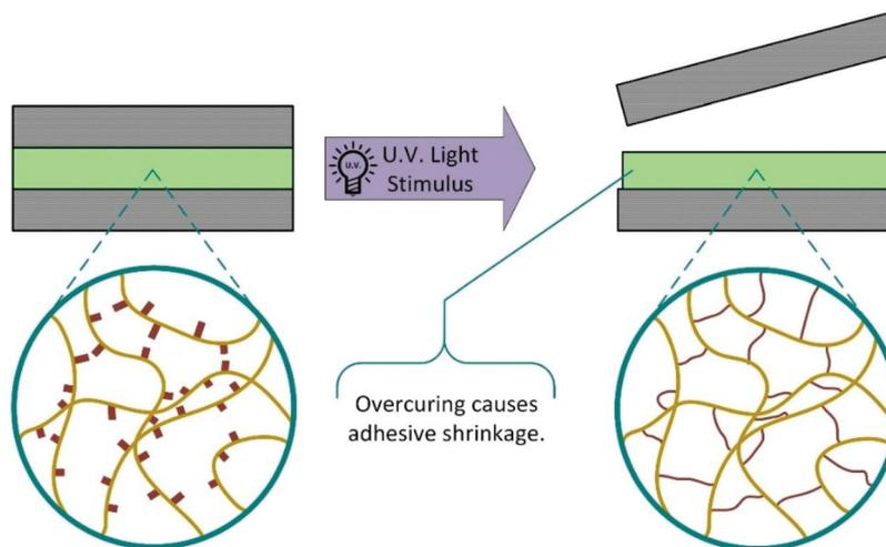
**Scheme 3** Schematic representation of photoinduced overcuring causing adhesive failure.
