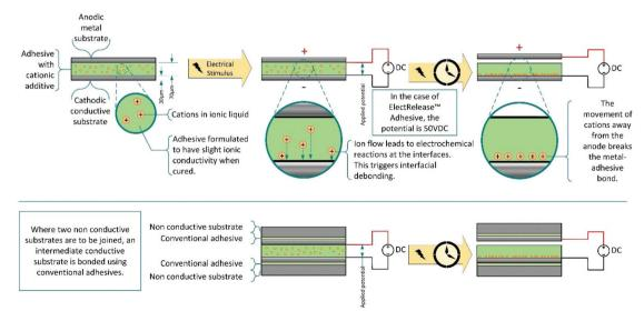
Scheme 14 Schematic representation of electrically debondable adhesives.
