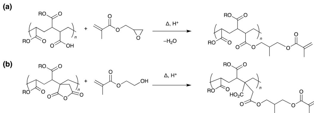
**Scheme 4** Representative examples of side chain functionalisation of acrylic copolymers with methacrylate residues.<sup>9,15</sup>
