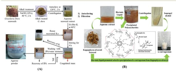
Fig. 5 (A) Selective precipitation of agarose using bio-ionic liquid (reproduced from ref. 110 with permission from The Royal Society of Chemistry). (B) Bio-ionic liquid-promoted selective precipitation from seaweed extracts (reproduced from ref. 61 with permission from Elsevier).
