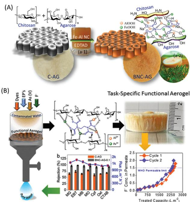
**Fig. 8** (A) Fabrication of iron and aluminium based composite functionalised aerogel and (B) performance of the aerogel membrane for the separation of dyes, pharmaceutical drugs, surfactants and fluoride ions from an aqueous medium.<sup>141</sup>
