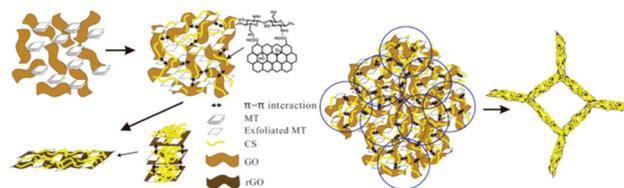
Fig. 6 Schematic representation of the fabrication of a composite hydrogel with a porous structure.<sup>140</sup>
