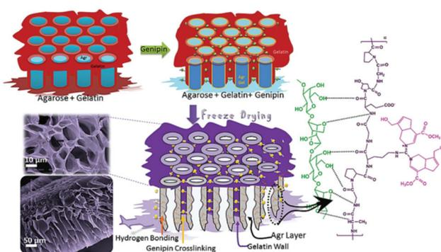
Fig. 11 Schematic representation of genipin crosslinked agarose-gelatin hydrogel formation and superhydrophilic, porous biobased aerogel membrane formation.<sup>211</sup>
