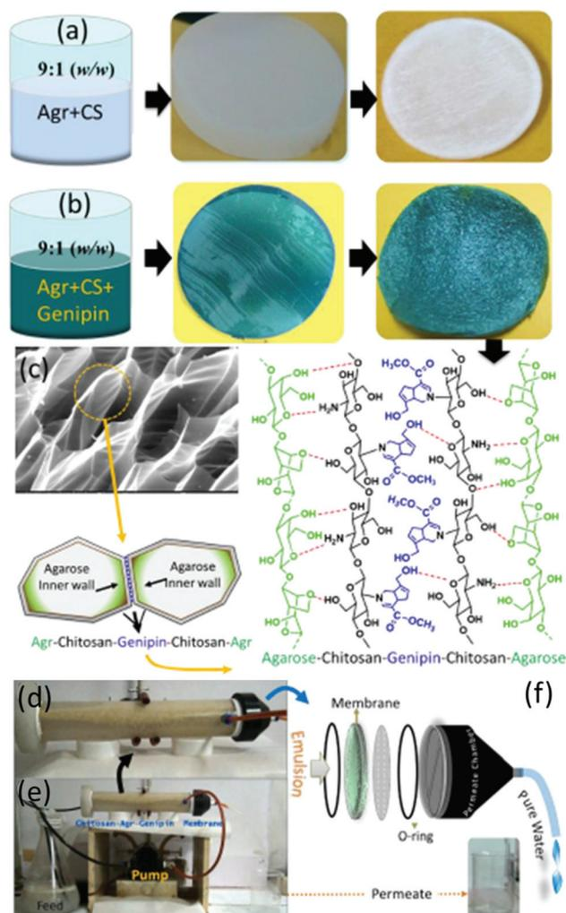
Fig. 9 (a–c) Schematic and digital images of highly crosslinked, superhydrophilic agarose/chitosan aerogel. (d–f) Cross-flow membrane filtration of crude oil based emulsion separation.<sup>210</sup>
