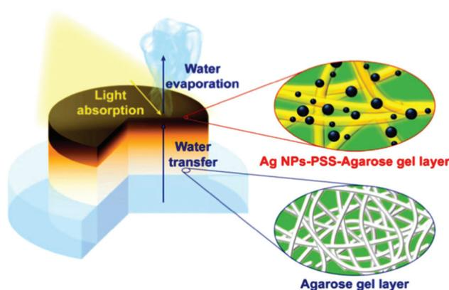
Fig. 12 Schematic representation of agarose-based double-layer hydrogel for solar-assisted water evaporation.<sup>295</sup>
