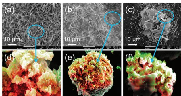
Fig. 15 (a–c) SEM images and (d–f) elemental mapping of graphene-like carbon material obtained by treating *Sargassum tenerrimum* with iron, tin and zinc based DES, respectively.<sup>332</sup>
