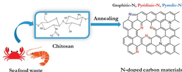
Fig. 14 Pyridinic, pyrrolic and graphitic N-doped carbonaceous materials derived from chitosan.<sup>347</sup>
