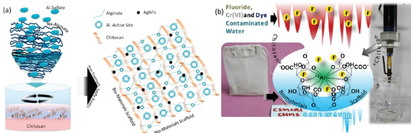
**Fig. 10** (a) Schematic representation of the preparation of an aluminium-composite-impregnated sodium alginate and chitosan-based biomaterial scaffold. (b) Shows the application of the bio-composite for the separation of dyes, Cr(VI) and fluoride through a teabag model and a continuous flow method.<sup>277</sup>
