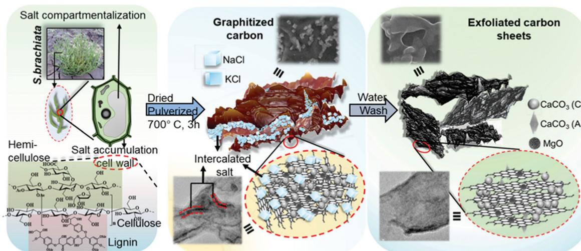
Fig. 13 Schematic representation of the complete process for the fabrication of porous carbon nanosheets from *Salicornia brachiata* biomass.<sup>340</sup>
