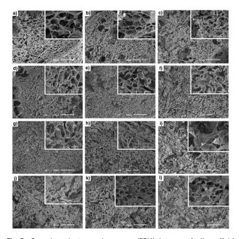
Fig. 2 Scanning electron microscopy (SEM) images of all scaffolds (freeze-dried condition): (a) to (h) (H $_1$  to H $_8$ , respectively) are related to samples produced by blending two biopolymers, while the images (i) to (l) (H $_9$  to H $_{12}$ , respectively) are from the biomaterials produced by blending three marine biopolymers. All images at the magnification of x50/500  $\mu$ m, x100/100  $\mu$ m, and x500/50  $\mu$ m.
