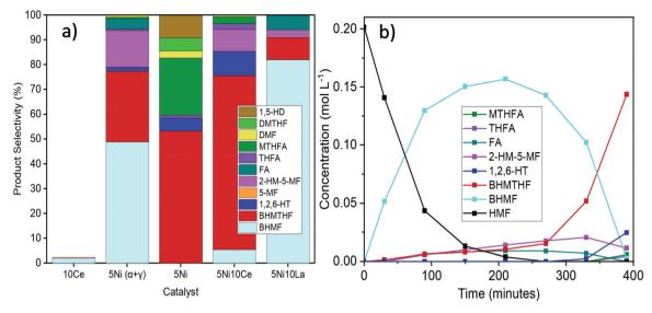
Fig. 1 (a) Comparison of product selectivity between activity tests using different supports and dopants (reaction conditions: 200 °C, 50 bar of  $H_2$ , 6 hours, THF as the solvent). (b) Demonstration of the product selectivity as a function of time with the 5Ni10Ce catalyst.
