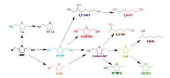
Scheme 1 Proposed reaction network of HMF hydrogenation.
