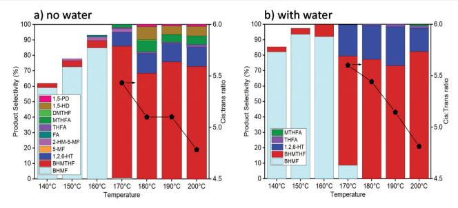
Fig. 2 Activity tests with the reaction temperature from 140-200 °C with pure THF (a) and 5 vol% H<sub>2</sub>O in THF (b) as the solvent (reaction conditions: 10Ni15Ce catalyst, 50 bar of H<sub>2</sub>, 3 hours).
