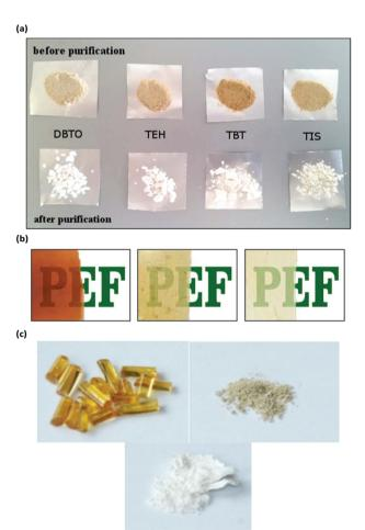
Fig. 1 The appearance of PEF (a) prepared with different catalysts after 2 h melt polycondensation at 230 °C, 152 reproduced by permission of The Royal Society of Chemistry, (b) prepared with different catalysts TBT, ZnAcO, and Al(acac)<sub>3</sub>, reprinted (adapted) with permission from ref. 153 (Copyright 2019 American Chemical Society), (c) derived from polycondensation (left) and ROP (middle and right) (CC BY 4.0) (adapted with permission from ref. 154).
