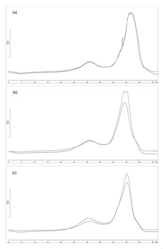
Fig. 5 DSC curves for (a) Sm MIX, (b) Sm MIX after SHF at LSR 6 g  $g^{-1}$ , and (c) Sm MIX after SHF at LSR 4 g  $g^{-1}$ .
