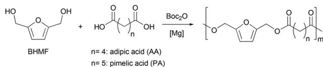
Scheme 2 Copolymerisation of BHMF and linear aliphatic diacids.
