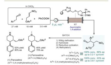
Scheme 12 Combined batch and flow synthesis of (+)-paroxetine and (+)-femoxetine.<sup>89</sup>
