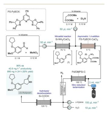
Scheme 3 Multistep telescoped continuous flow asymmetric synthesis of (S)-rolipram.<sup>50</sup>
