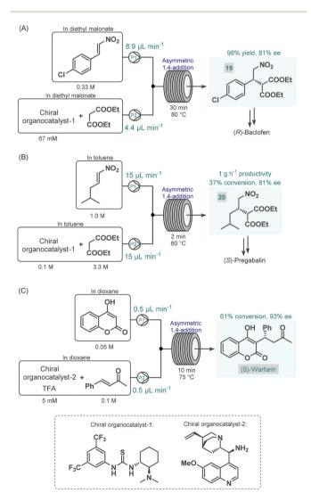
Scheme 8 Enantioselective synthesis of GABA-derived API precursors as well as (S)-warfarin in homogenous organocatalytic flow processes.<sup>73</sup>
