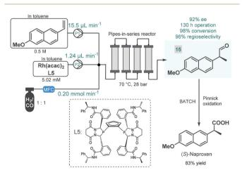
Scheme 6 Continuous flow enantioselective synthesis of a chiral naproxen precursor. <sup>62</sup>
