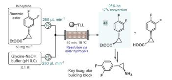
Scheme 18 Continuous flow synthesis chiral ester 43 via biocatalytic resolution.<sup>111</sup> (TLL = lipase from *Thermomyces lanuginosus*).
