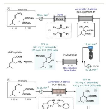
**Scheme 5** Continuous flow asymmetric synthesis of chiral pregabalin precursors. <sup>59,60</sup>
