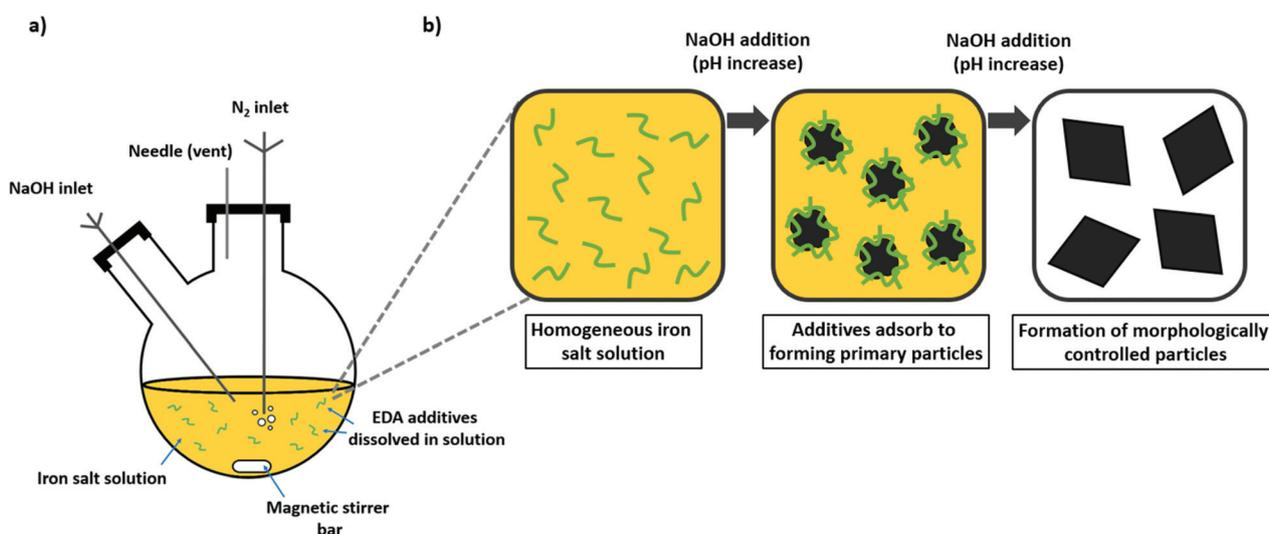
**Fig. 1** (a) Schematic of the experimental setup for an RTCP reaction containing an organic additive or protein *in vitro*. (b) The reaction progression on addition of NaOH is shown, with the role of additives adsorbing to the surface of forming primary particles, and finally the production of morphologically controlled particles.
