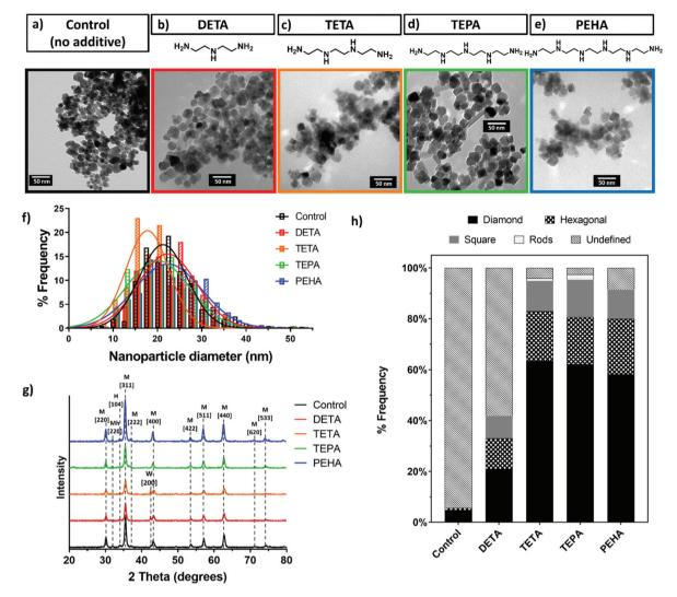
Fig. 2 MNP analysis: Representative TEM images of nanoparticles formed with the addition of various additives. (a) Control (no additive); (b) DETA; (c) TETA; (d) TEPA; (e) PEHA, with scale bars and additive structure. (f) Frequency distribution histogram of particles; (g) annotated XRD data where M = magnetite, Mh = maghemite, H = hematite, and W = wüstite. (h) Shape distribution of particles from TEM images. All scale bars are 50 nm.
