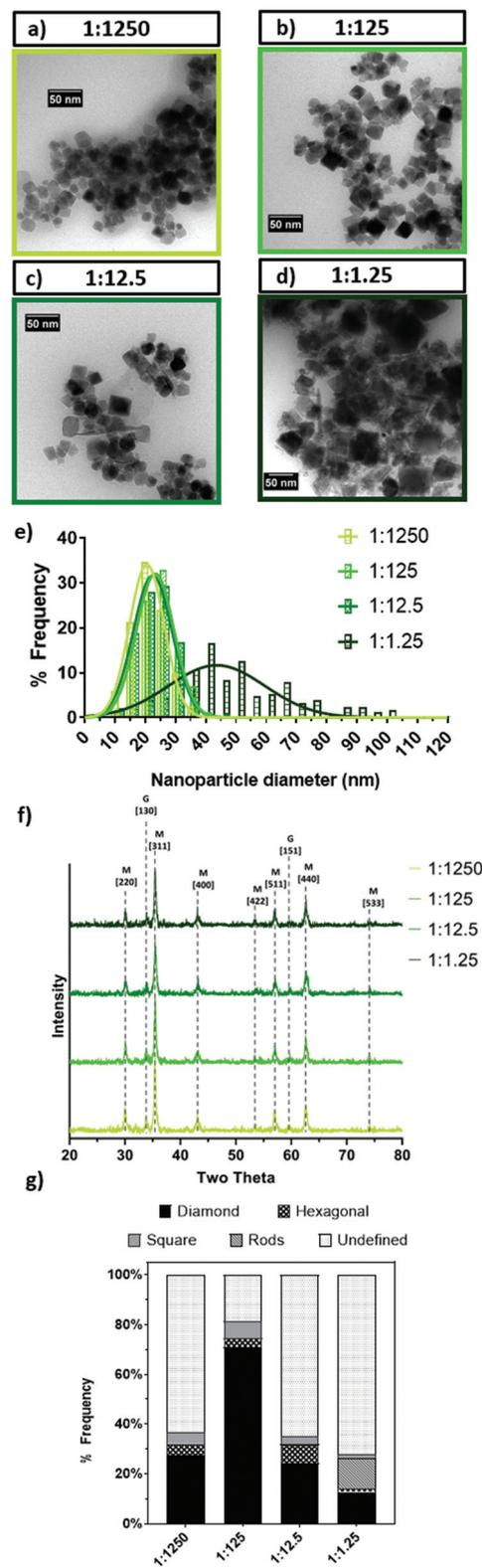
**Fig. 8** MNP analysis: Representative TEM images of nanoparticles formed with varying TEPA:iron ion ratios. (a) 1 : 1250; (b) 1 : 125; (c) 1 : 12.5; (d) 1 : 1.25; (e) frequency distribution histogram of particles; (f) annotated XRD data where M = magnetite and G = goethite; (g) shape distribution of particles from TEM images. All scale bars are 50 nm.
