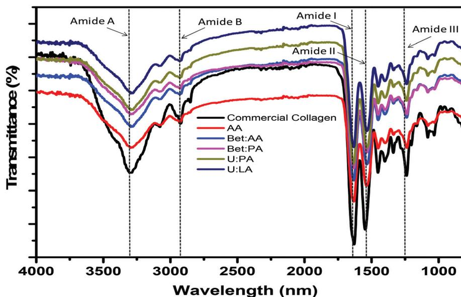
Fig. 3 FTIR spectra of commercial collagen and collagen type I extracted using aqueous solutions of AA and DES. FTIR spectra were collected in the range of 4000–250  $\text{cm}^{-1}$  by accumulating 256 scans, and with a resolution of 4  $\text{cm}^{-1}$  at room temperature.
