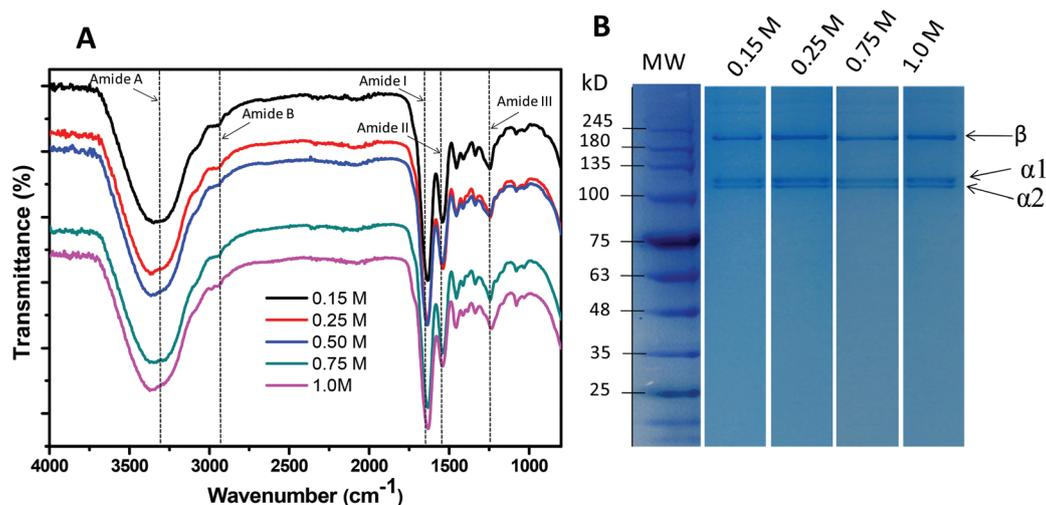
Fig. 9 Characterization of collagen extracted from the skin of codfish using U : LA (1 : 2) at different concentrations: (A) FTIR spectra; (B) SDS-PAGE.
