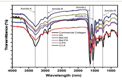
Fig. 3 FTIR spectra of commercial collagen and collagen type I extracted using aqueous solutions of AA and DES. FTIR spectra were collected in the range of 4000–250 cm<sup>-1</sup> by accumulating 256 scans, and with a resolution of 4 cm<sup>-1</sup> at room temperature.
