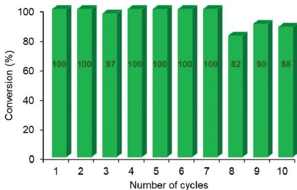
**Fig. 3** Testing the reusability of the AgBi-HM catalyst in the decarboxylation of 2-nitrobenzoic acid. Selectivity was 100% in all reactions. (Reaction conditions: 0.15 M substrate concentration, 5 mol% catalyst, 15 mol% of KOH as base, DMF as solvent, 110 °C, 24 h reaction time.).
