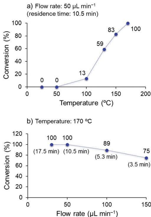
**Fig. 4** Investigation of the effects of the reaction temperature (a) and residence time (b) in the AgBi-HM-catalyzed decarboxylation of 2-nitrobenzoic acid in a continuous flow reactor. (Reaction conditions: 0.1 M substrate concentration, 15 mol% of KOH as base, MeCN as solvent.).
