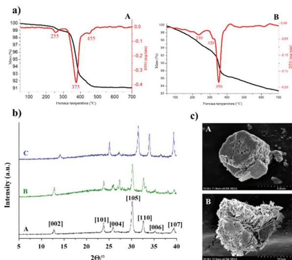
**Fig. 6** (a) Thermal behaviour of used AgBi-HM samples: sample used in flow scale-out (A), sample used in batch recycling experiment (B). (b) Comparison of the X-ray patterns of various AgBi-HM samples: as-prepared sample (A), sample used in batch recycling experiments (B), sample used in flow scale-out (C). (c) SEM images: as-prepared AgBi-HM sample – micrograph taken from ref. 41 (A), AgBi-HM sample used in flow scale-out (B).
