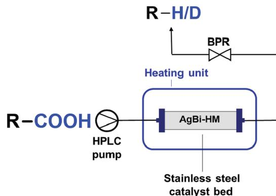
Fig. 1 Experimental setup for the continuous flow experiments.
