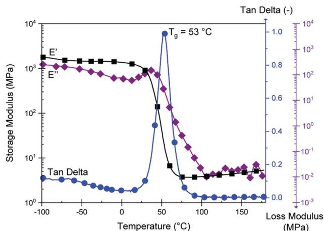
Fig. 5 DMTA data ( $-100 \text{ }^\circ\text{C}$  to  $180 \text{ }^\circ\text{C}$ , 1 Hz, 0.1% strain) of cured CBDA-2/ELO thermosets using a fixed COOH/oxirane group-ratio of 0.8 (the symbols are intended to help differentiate the curves and do not represent the sole data points).
