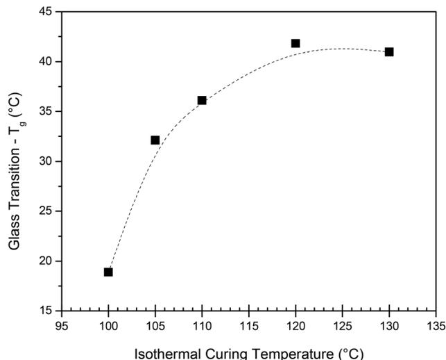
Fig. 3 Obtained  $T_g$  of samples cured for 2 h at different isothermal curing temperatures. The  $T_g$  was determined immediately after the isothermal curing of the samples by cooling and heating the samples at 10 K min<sup>-1</sup>.
