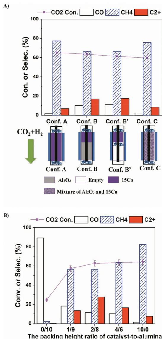
**Fig. 2** Influence of catalyst-bed configuration (a) and catalyst-to-alumina ratio over Conf. B (b) on the CO<sub>2</sub> conversion and product distributions in the CO<sub>2</sub> hydrogenation over 15Co catalyst coupled with DBD plasma at the furnace temperature of 250 °C. Reaction conditions: 20 v% CO<sub>2</sub>–60 v% H<sub>2</sub> in Ar balance, H<sub>2</sub>/CO<sub>2</sub> = 3, flow rate = 20 mL min<sup>-1</sup>, P = 1 atm, voltage = 13.6 kV, frequency = 23.5 kHz, plasma power = 4 W.
