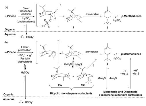
Fig. 10 (a) Slow hydrolysis of α-pinene in the absence of Me<sub>2</sub>S proceeds *via* an undissociated acid mechanism. <sup>45</sup> (b) Faster hydrolysis of α-pinene occurs through a more dissociated acid mechanism caused by formation of terpene sulfonium salts that act as surfactants to increase mixing at the interfacial layer to create a more acidic microenvironment that increases the overall rate of the ACRO reaction.  $HSO_4^-$  counterions of carbenium species omitted for clarity.
