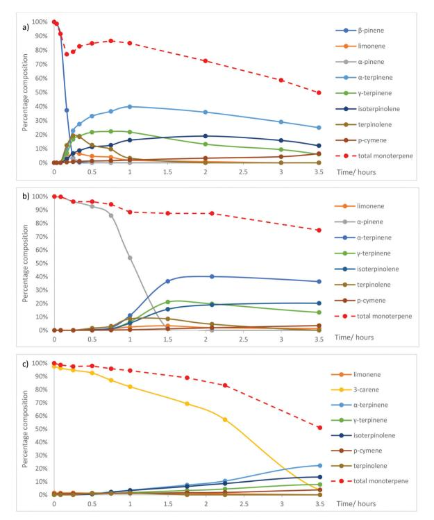
Fig. 4 Changes in the ratio of the mixtures of p-MeDs when (a) β-pinene; (b) α-pinene; and (c) 3-carene were reacted with 6 M aq.  $H_2SO_4$  and 5 mol%  $Me_2S$  at 90 °C over time.
