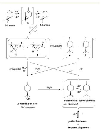
Fig. 6 Mechanism of the ACRO reaction of 3-carene to afford isolimonene and isoterpinolene. HSO<sub>4</sub> counterions of carbenium species omitted for clarity.
