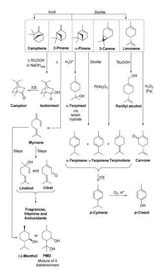
**Fig. 1** A representative range of scalable catalytic reactions that can be used to transform purified monoterpenes from turpentine into valuable biorenewable chemical products on an industrial scale.
