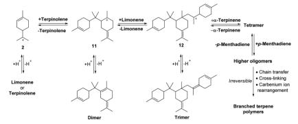
Fig. 8 Reversible cationic polymerisation of monomeric/oligomeric carbenium species using different p-MeD donors affords a complex mixture of oligomeric and polymeric terpenoid species over time. Representative oligomerisation process shown for limonene, terpinolene and α-terpinene participating as p-MeD monomers in the oligomerisation process. HSO<sub>4</sub> $^-$  counterions of carbenium species omitted for clarity.
