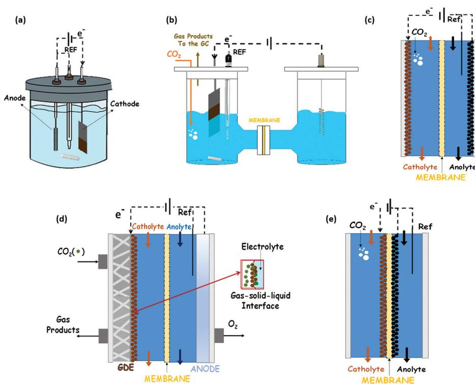
Fig. 5 Schematic concepts of (a) traditional 3-electrode cell, (b) H-type cell, (c) two compartments cell, (d) Gas Diffusion Electrode cell and (e) Membrane Electrode Assembly for electrochemical  $CO_2$  reduction reactions.
