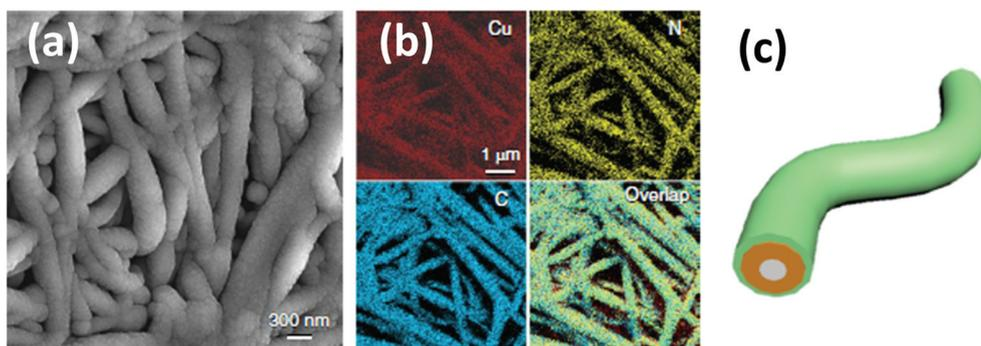
**Fig. 9** Structural and compositional analyses of the 34% N-C/Cu catalyst on PTFE. (a) Low-magnification SEM image of the 34% N-C/Cu catalyst on PTFE. (b) EDX elemental mapping of Cu, N and C for the 34% N-C/Cu catalyst on PTFE. (c) Scheme of the cross-sectional structure of a N C/Cu/PTFE nanofibre. The white, orange and green layers represent PTFE, Cu and N-C, respectively. Reproduced from ref. 90 with permission of nature energy.
