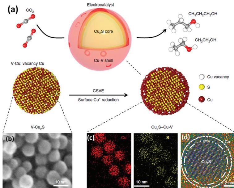
**Fig. 10** Catalyst design and structural characterization. (a) Schematic illustration of  $\text{Cu}_2\text{S-Cu-V}$  electrocatalyst design for production of multi-carbon alcohols from  $\text{CO}_2$  reduction. (b) TEM showing the uniform size. (c) EDS mapping showing the homogeneous distribution of Cu and S. (d) high-resolution TEM. Reproduced from ref. 91 with permission of nature catalysis.
