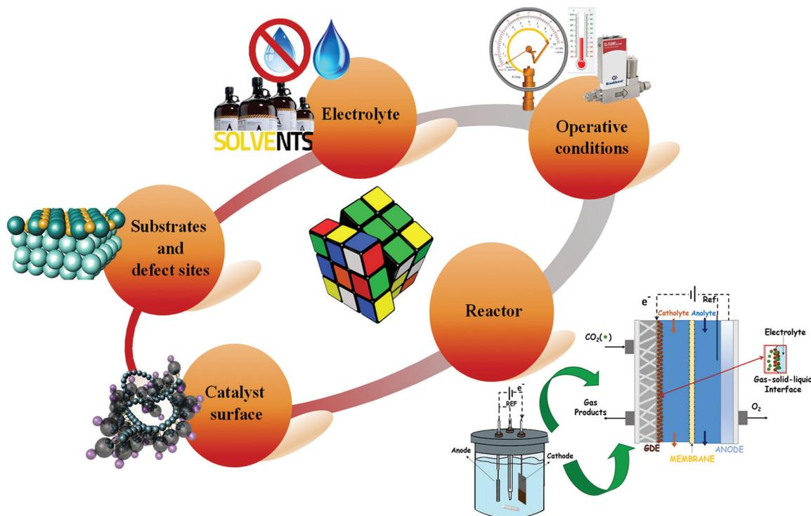
Fig. 3 Factors influencing the electrochemical CO<sub>2</sub> conversion performance.
