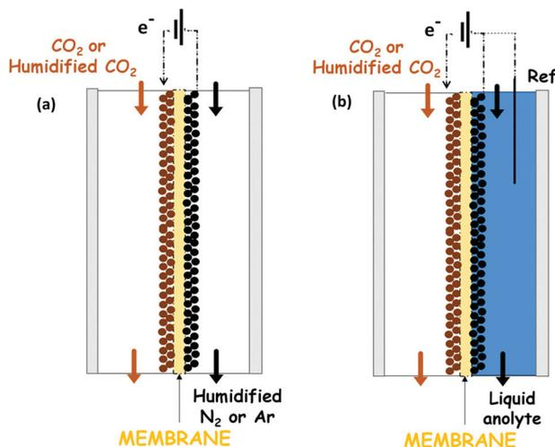
Fig. 12 Representation of the most popular catholyte-free configuration, in continuous flow, for the electrochemical CO<sub>2</sub> reduction: (a) solvent-less cell configuration, (b) liquid anolyte cell configuration.
