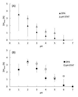
Fig. 1 Degree of hydrolysis measured after 3 min of gastric digestion (DH $_{3min}$ ) at different pH for EWP (A) and CA (B), as estimated from (i) the OPA method on the end samples of the gastric digestion lasting 3 min (filled symbols) and (ii) the pH-STAT method at 3 min of the gastric digestion lasting 2 h (open symbols). Data represent mean  $\pm$  SD over 3 replicates.
