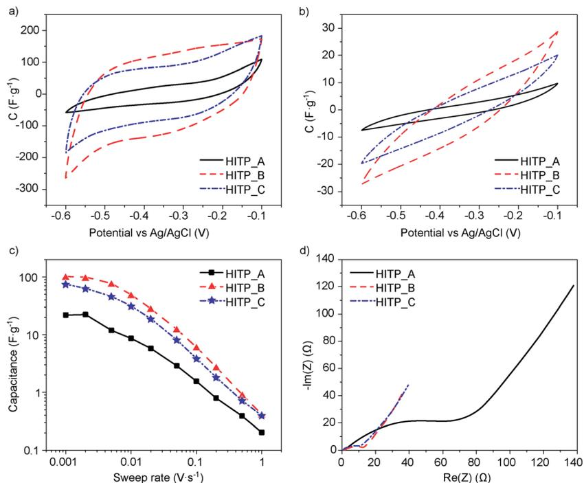
Fig. 2 Results of characterization of 3 electrode cells prepared from the three different  $\text{Ni}_3(\text{HITP})_2$  batches. Cyclic voltammetry at 1  $\text{mV s}^{-1}$  (a) and 100  $\text{mV s}^{-1}$  (b). Capacitance retention as a function of the voltage sweep rate (c). Electrochemical impedance spectra (d).
