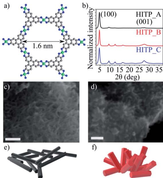
Fig. 1  $\text{Ni}_3(\text{HITP})_2$  molecular structure as a ball-and-stick model, where carbon is grey, nickel is green and nitrogen is blue (a), normalized intensity PXRD patterns of the three  $\text{Ni}_3(\text{HITP})_2$  batches (b), SEM micrographs of HITP\_A (c) and HITP\_B (d), where the scale bar is 200 nm, 3D schematics of the crystal morphology for HITP\_A (e) and HITP\_B (f) based on the arrangement seen in the SEM images; HITP\_C shows the same morphology as HITP\_B (Fig. S1†).
