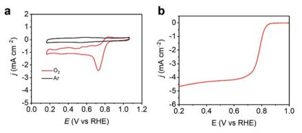
Fig. 7 (a) CVs of ZIF-EC1(Zn,Co) catalyst in 0.1 M KOH in an  $Ar/O_2$ -saturated solution. (b) LSV curves of ZIF-EC1(Zn,Co) catalyst in 0.1 M KOH in an  $O_2$ -saturated solution at 1600 rpm.
