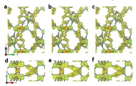
Fig. 6 Electrostatic potential maps calculated based on datasets 1-8 merged by (a and d) XSCALE, (b and e XPREP, and (c and f) AIMLESS. The refined structural model is superimposed in the map and used for calculating the structure factor phases. All electrostatic potential maps are drawn at the same contour level, which is the  $2\sigma$  level of M\_ABC dataset, and equals to an isosurface level  $d_{\rm iso}=0.811$ . Atom color codes: grey: C; blue: N; red: O; cyan: Zn.
