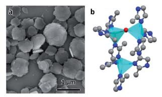
Fig. 1 (a) SEM image of ZIF-EC1 crystals. (b) The structural model of ZIF-EC1. Cyan tetrahedra: Zn atoms; red spheres: O atoms; blue spheres: N atoms; grey spheres: C atoms.
