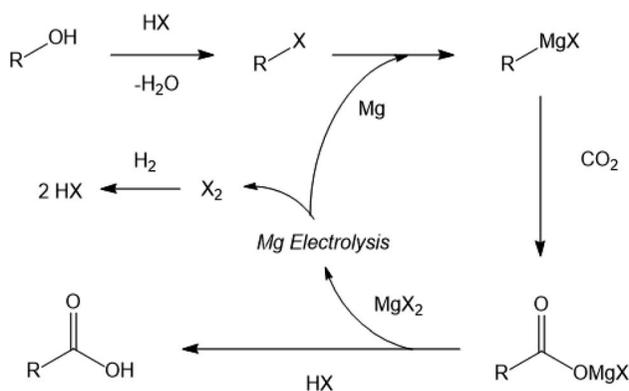
Fig. 1 Generalised scheme for the formation of a higher carboxylic acid from an alcohol and CO<sub>2</sub> using regenerable Grignard reagents.
