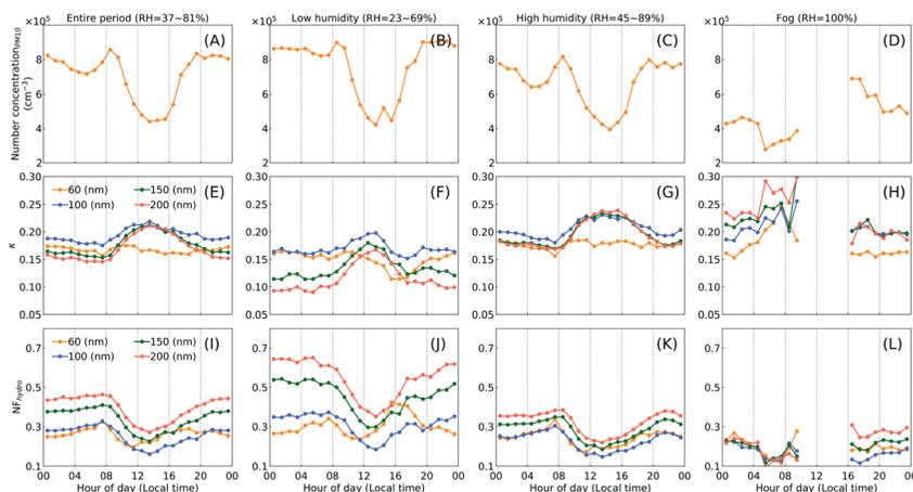
Fig. 8 Diel variations of particle number concentration in  $PM_{10}$  size range (top row), hygroscopicity parameter  $\kappa$  (second row) and number fraction of hydrophobic particles  $Nf_{\text{hydro}}$  for selected particle sizes (bottom row) averaged over the entire campaign and focus periods with different relative humidity (RH) conditions.
