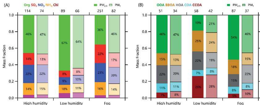
Fig. 5 Average (A) chemical composition of non-refractory PM<sub>2.5</sub> and PM<sub>1</sub>, and (B) OA composition during the focus periods with different relative humidity (RH) conditions. The numbers on the top of the figures are the average mass concentrations ( $\mu\text{g m}^{-3}$ ) for each period. Adopted and modified from Sun *et al.*<sup>19</sup>
