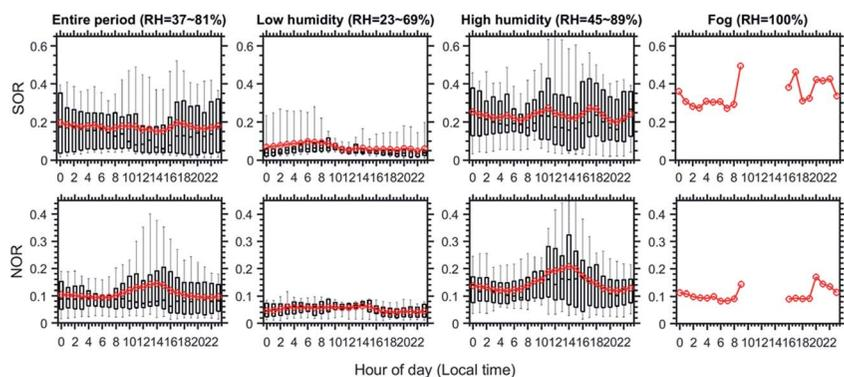
Fig. 4 Diel variations of the ratios of nitrate to nitrate plus  $\text{NO}_2$  (NOR) and sulfate to sulfate plus  $\text{SO}_2$  (SOR) averaged over the entire campaign and focus periods with different relative humidity (RH) conditions. The boxes and whiskers indicate percentiles (90th, 75th, 50th (median), 25th and 10th).
