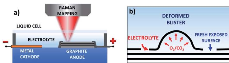
Fig. 1 (a) Schematic illustration of the Raman setup for *in situ* spectroscopic monitoring of the graphite exfoliation process; (b) schematic of the graphite exfoliation process during electrochemical oxidation.
